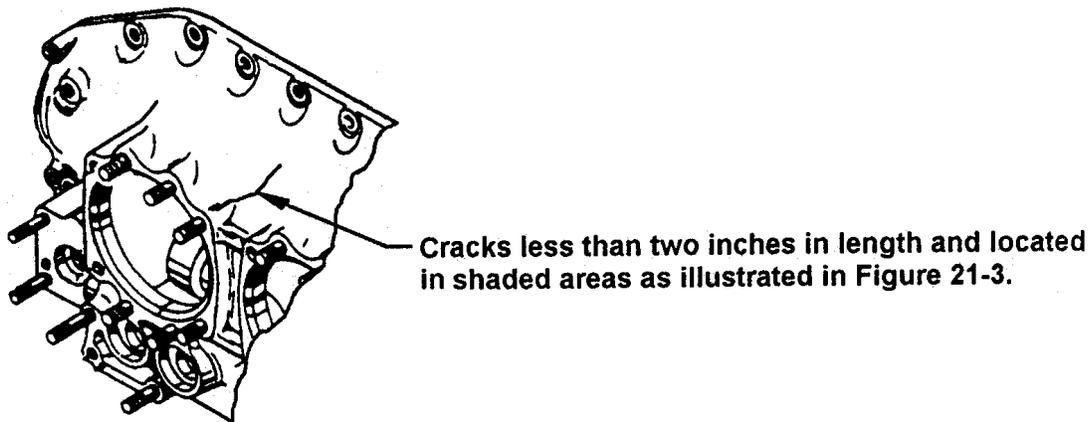
**FIGURE 21-2. INSPECTION OF CRANKCASE NON CRITICAL AREA**
