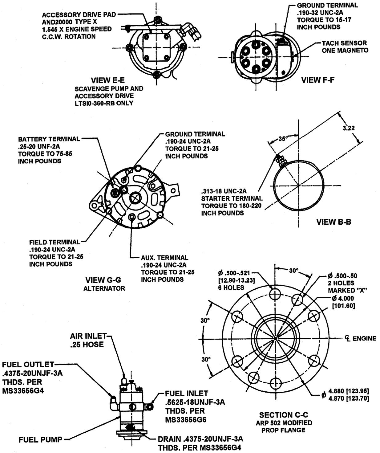
**FIGURE 6-1. INSTALLATION DRAWING (cont'd)**
