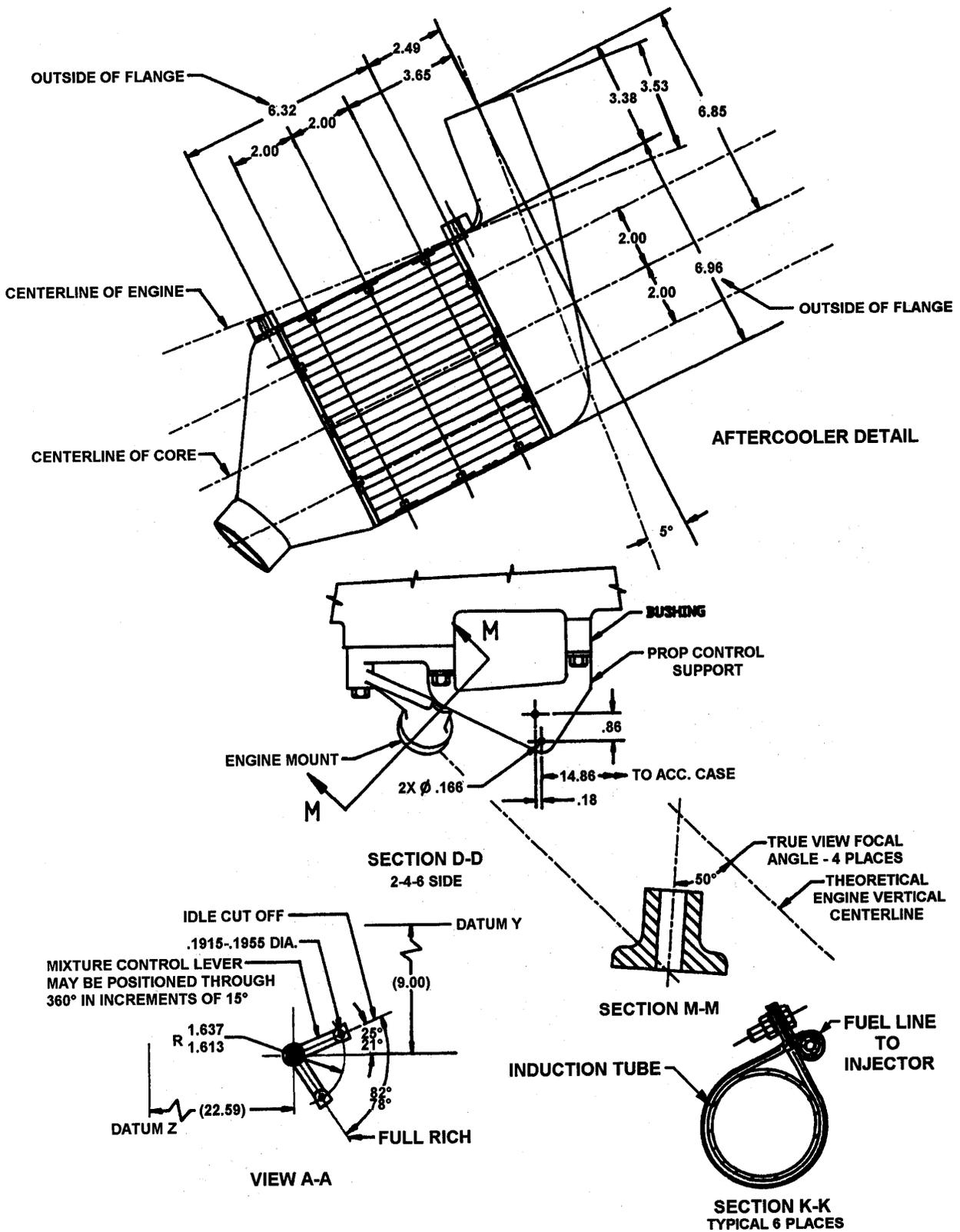
FIGURE 6-1. INSTALLATION DRAWING (cont'd)
