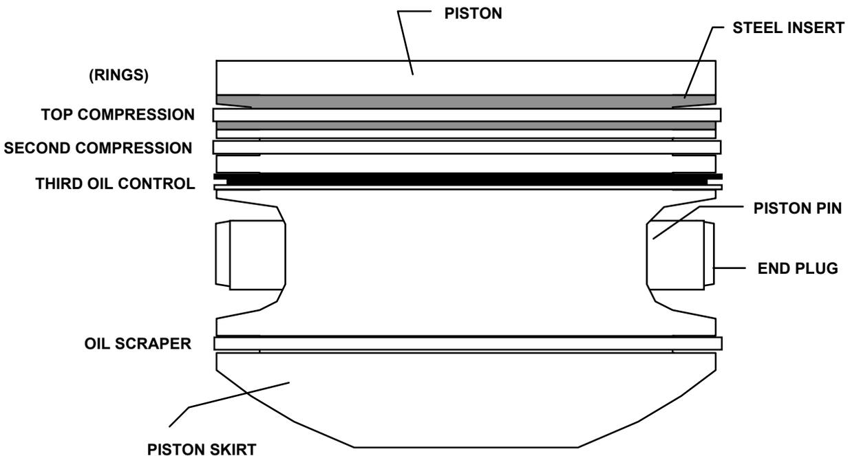
FIGURE 20-4. PISTON ASSEMBLY DISCRIPTION
