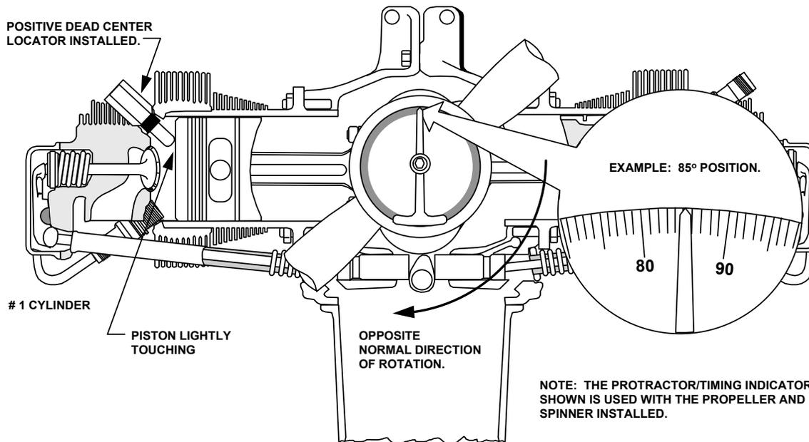
**FIGURE 12-5. TIMING POSITION STEP 2**
