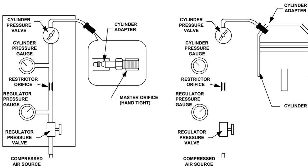
**FIGURE 20-10. DIFFERENTIAL PRESSURE TESTER CALIBRATION**
