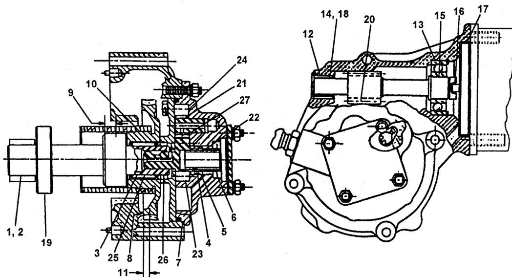
**FIGURE 17-3. STARTER ADAPTER FITS AND LIMITS
