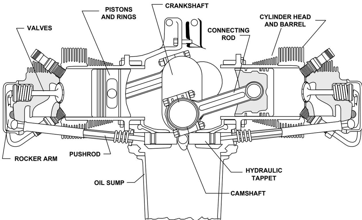
FIGURE 20-2. CYLINDER PISTON AND VALVE TRAIN
