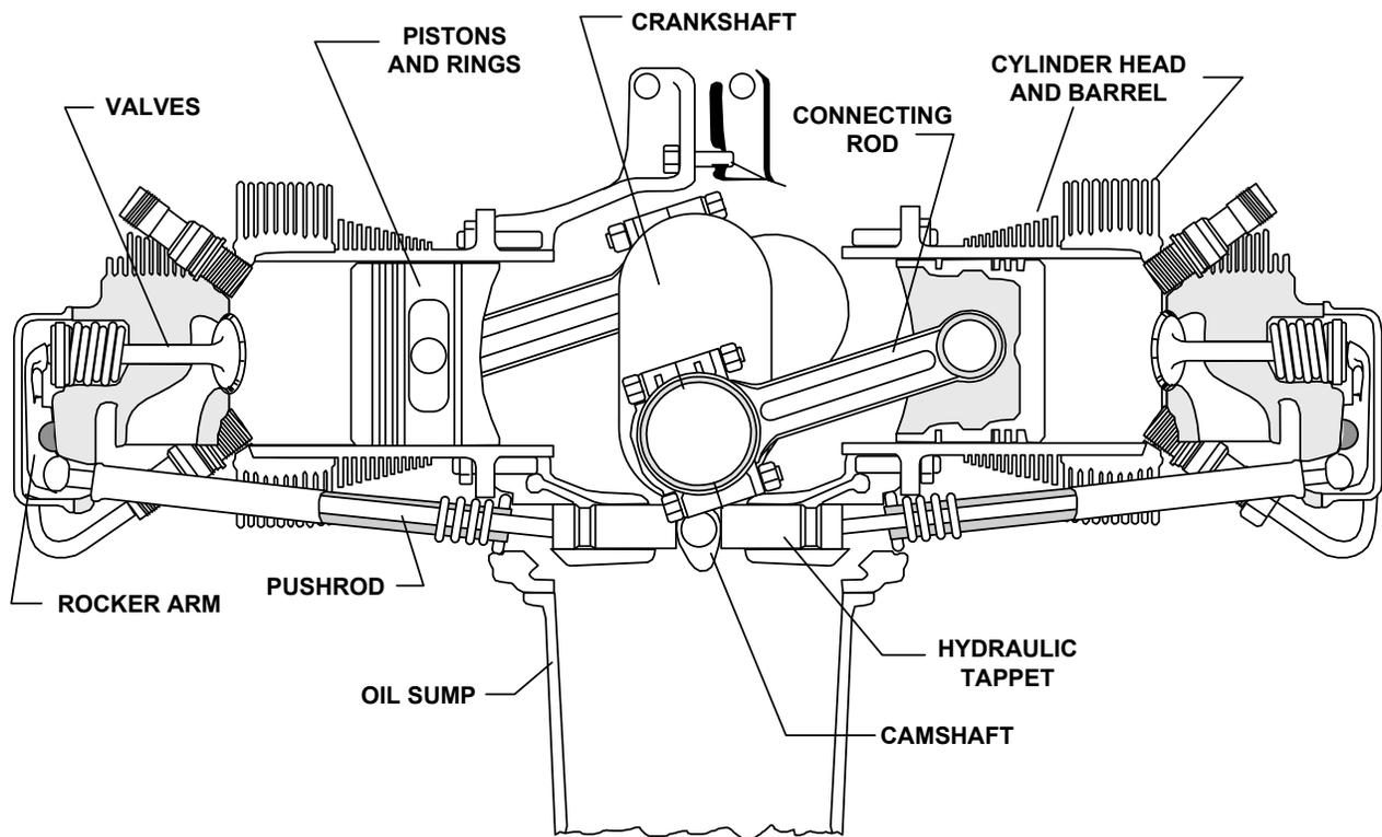
FIGURE 20-2. CYLINDER PISTON AND VALVE TRAIN
