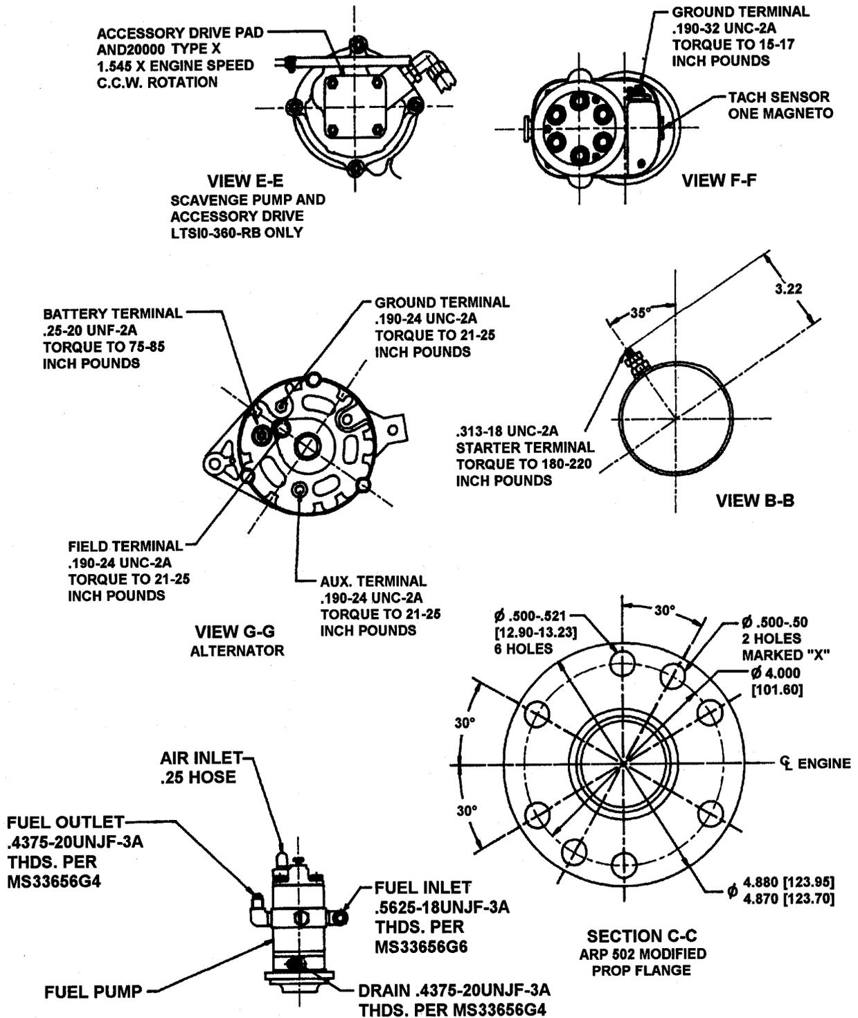
FIGURE 1-2. ENGINE DESCRIPTION L/TSIO 360-RB (Cont'd)
