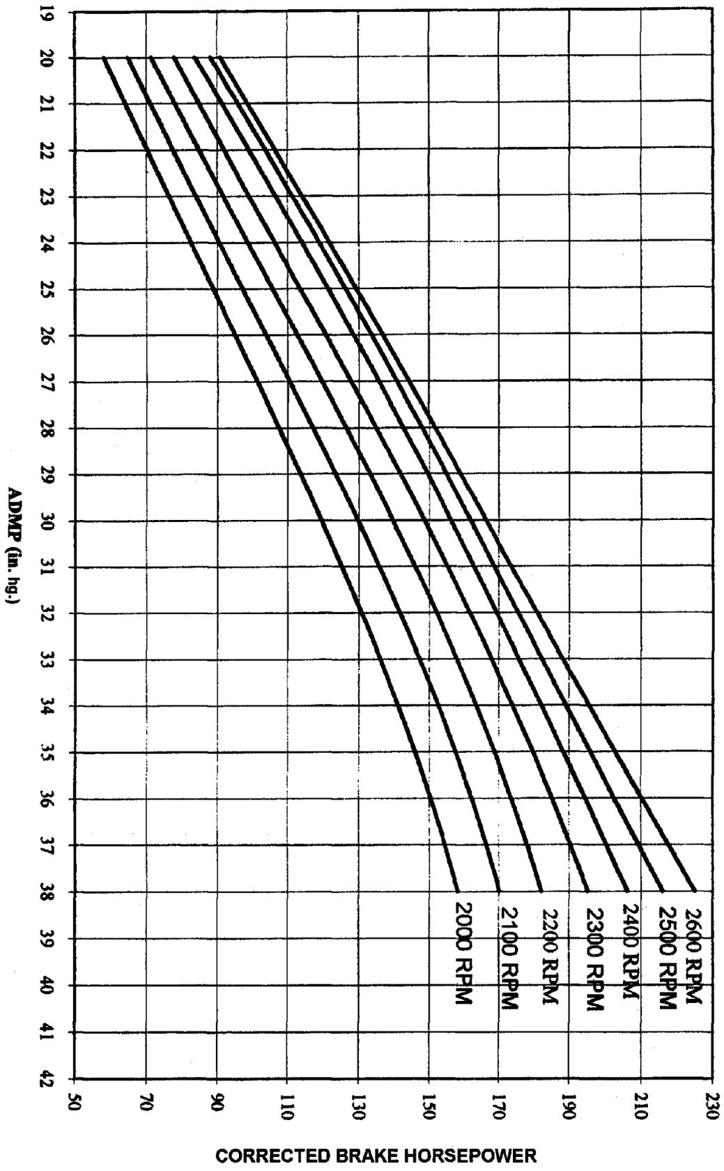
**FIGURE 23-6. CONSTANT SPEED SEA LEVEL PERFORMANCE CURVE**
