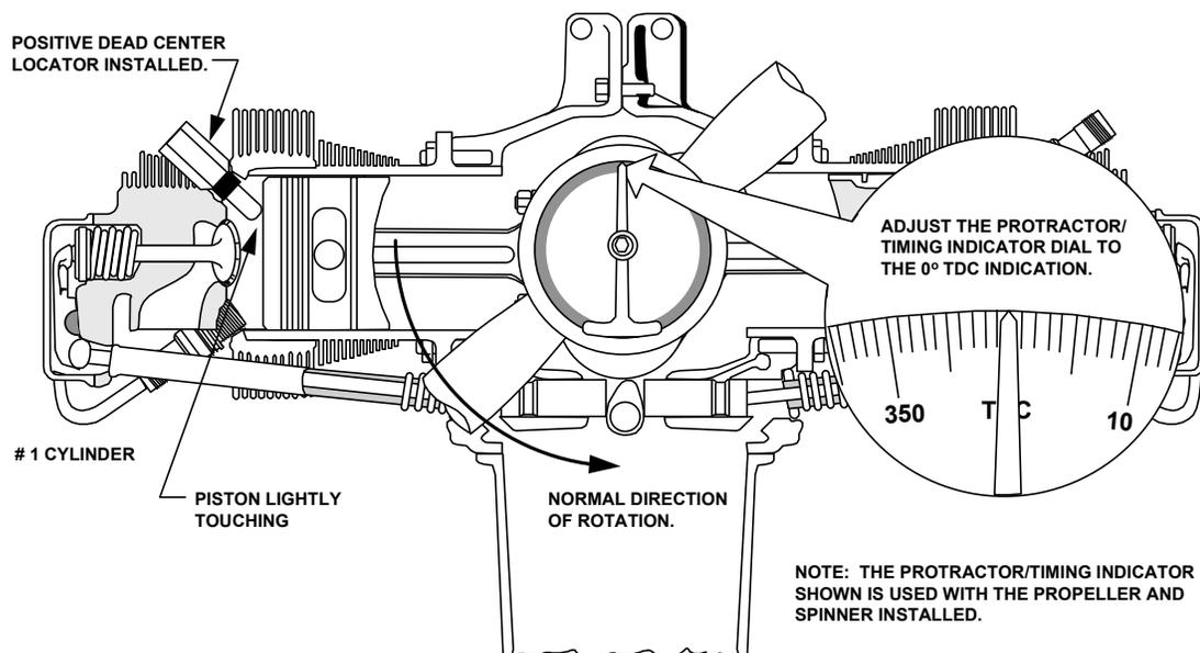
FIGURE 12-4 TIMING POSITION STEP 1
