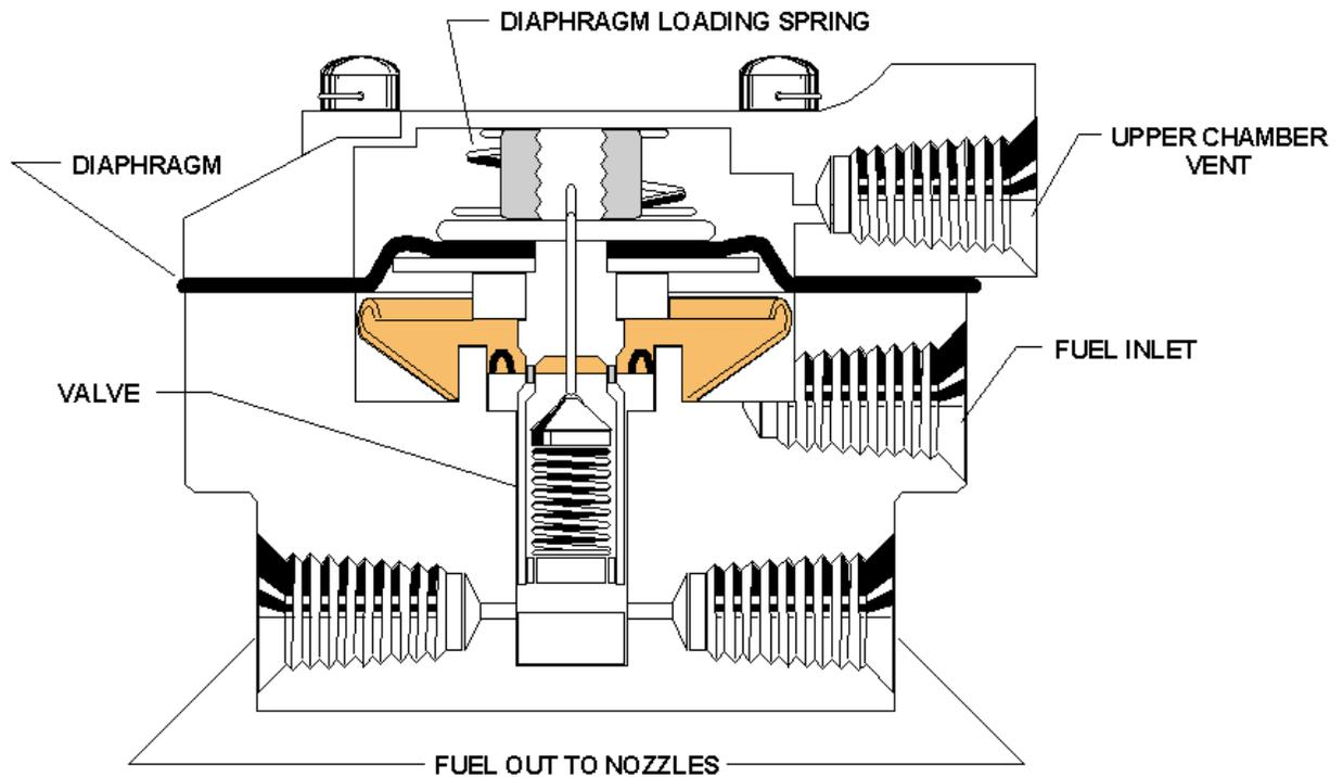
**FIGURE 13-2. GENERAL FUEL MANIFOLD VALVE DESCRIPTION**
