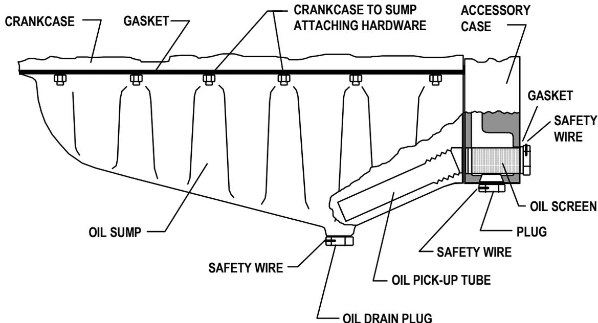
**FIGURE 19-5. OIL SUMP AND SUCTION TUBE DESCRIPTION**
