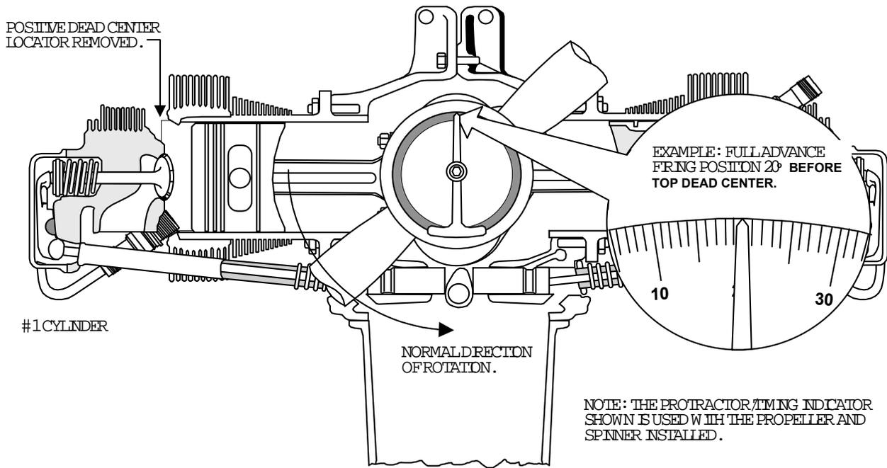
**FIGURE 12-5. TIMING POSITION STEP 5**
