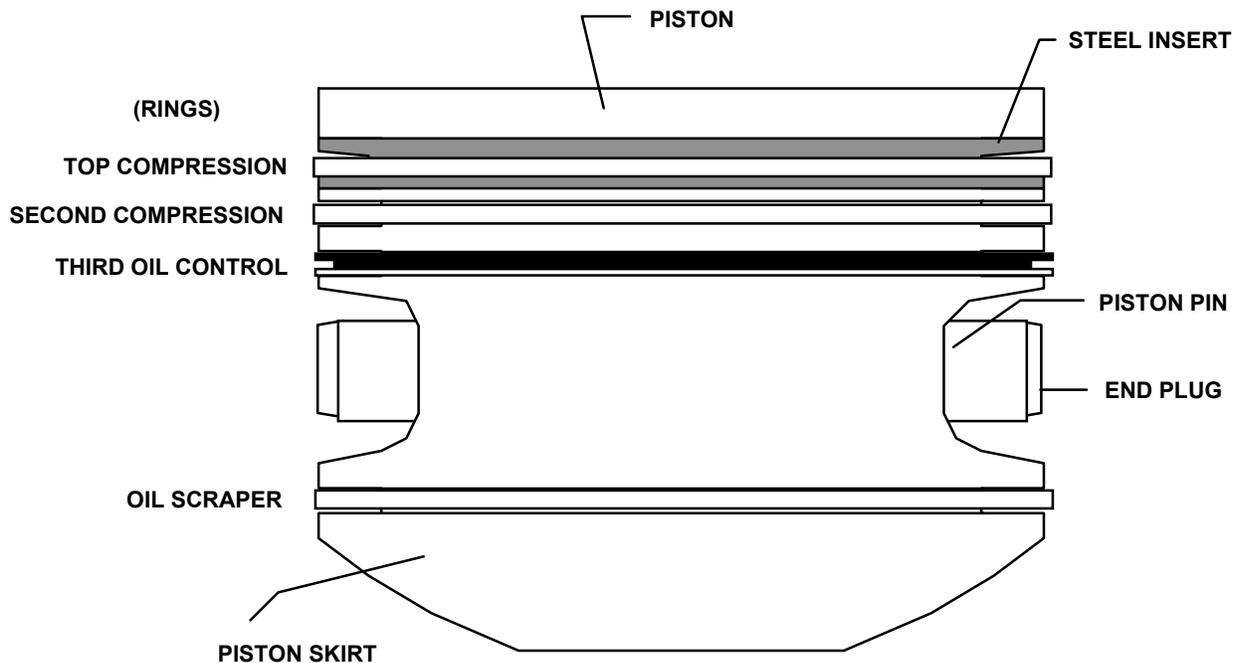
FIGURE 20-4. PISTON ASSEMBLY DISCRIPTION
