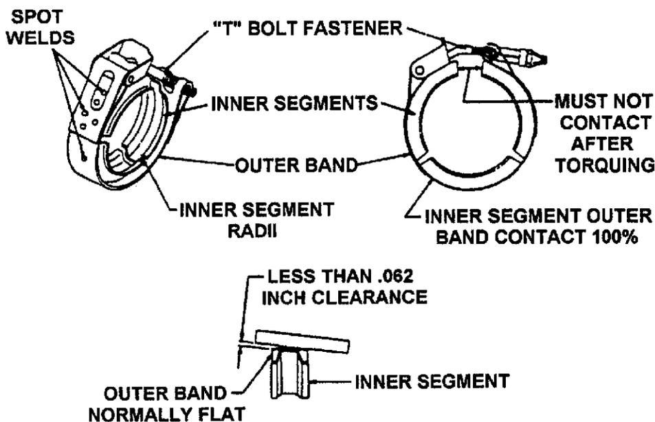
FIGURE 11-7. MULTI-SEGMENT "V" BAND CLAMP
