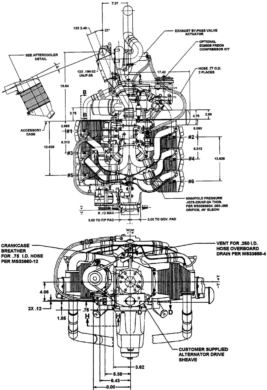
FIGURE 6-1. INSTALLATION DRAWING
