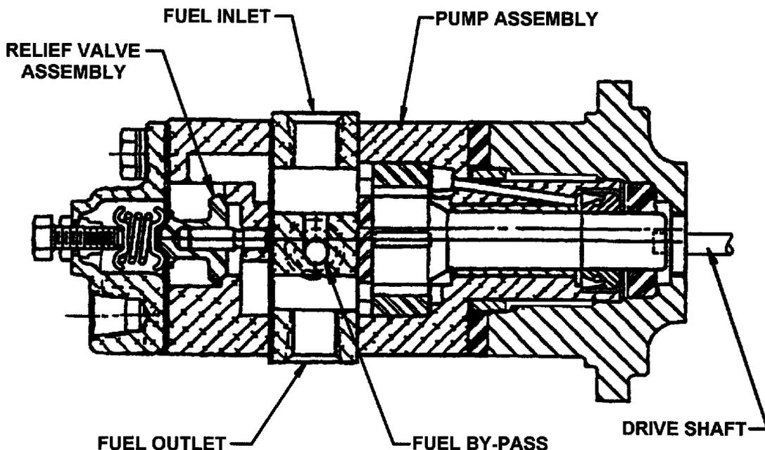
FIGURE 13-1. FUEL PUMP DESCRIPTION L/TSIO-360-RB
