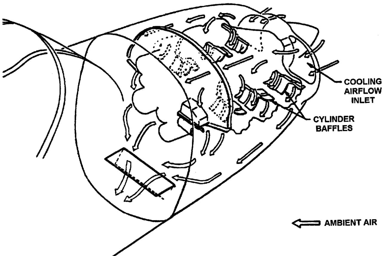
FIGURE 20-1. GENERAL ENGINE COOLING AIRFLOW DIAGRAM
