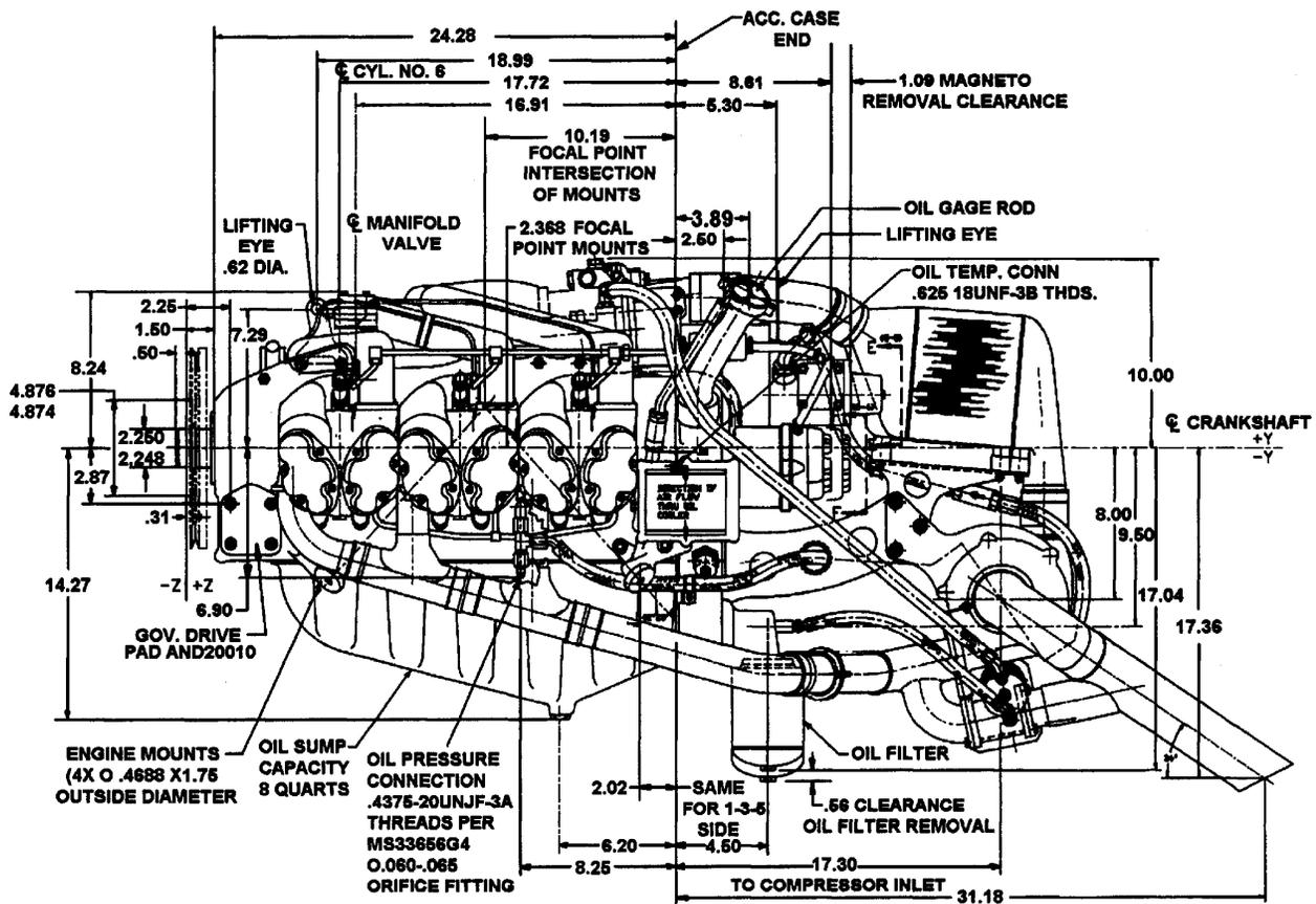
FIGURE 1-2. ENGINE DESCRIPTION L/TSIO 360-RB (Cont'd)
