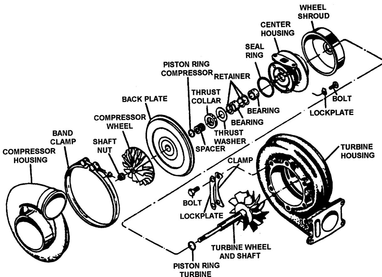
FIGURE 11-2. BASIC TURBOCHARGER
