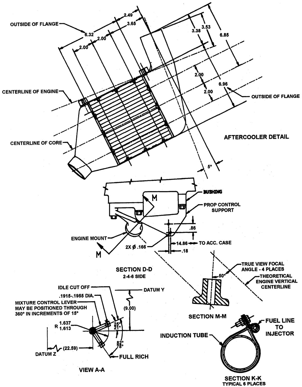
FIGURE 1-2. ENGINE DESCRIPTION L/T510 360-RB (Cont'd)
