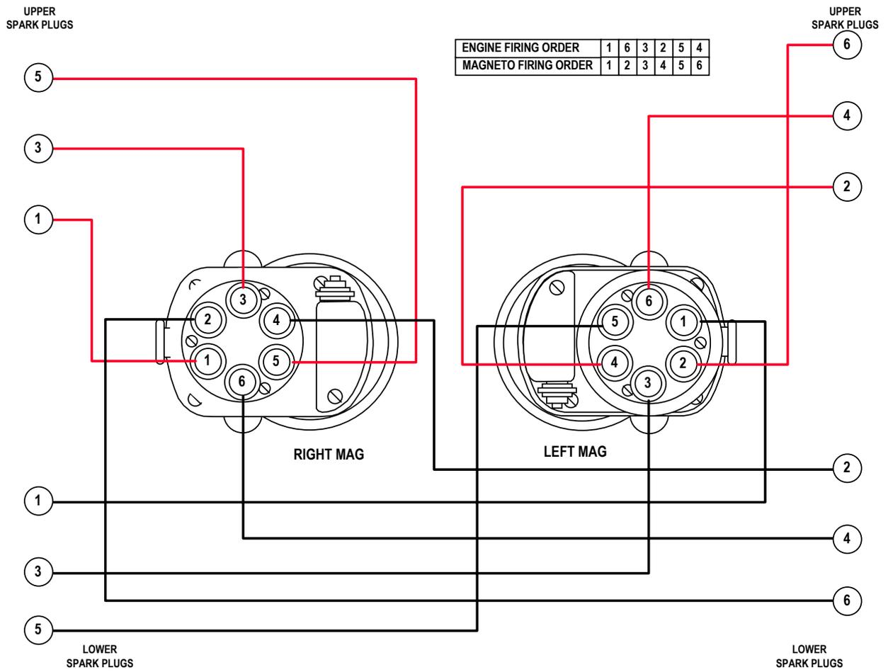
**FIGURE 12-10. IGNITION WIRING DIAGRAM**
