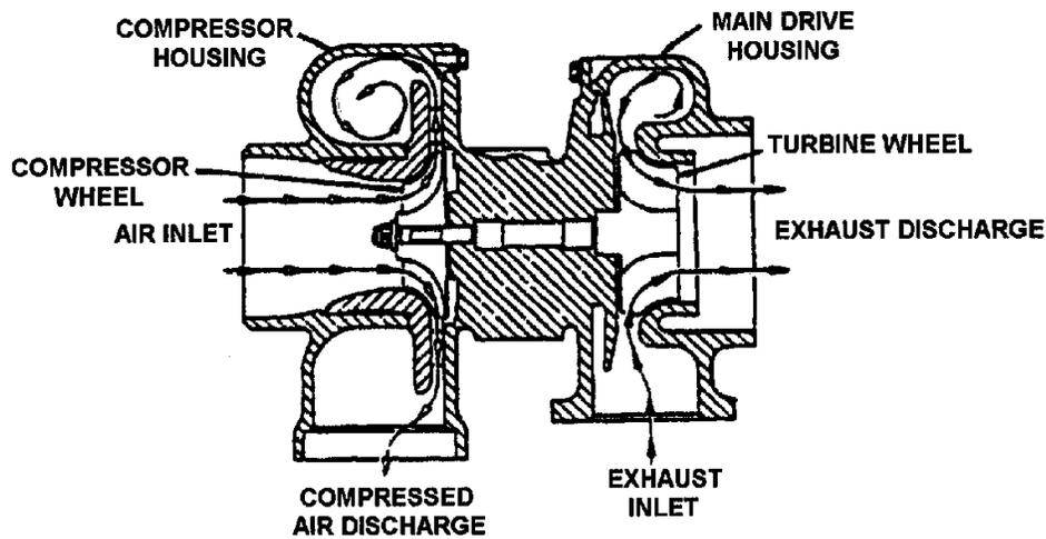
FIGURE 11-3. TURBOCHARGER SECTIONAL VIEW
