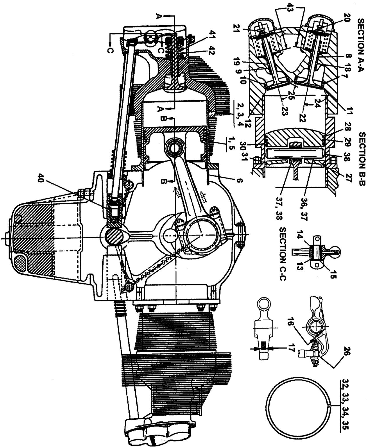
FIGURE 20-12. CYLINDER ASSEMBLY SERVICE LIMITS
