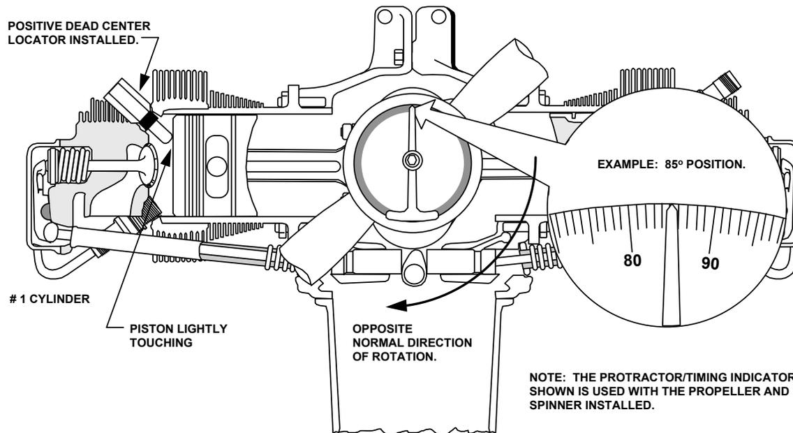
**FIGURE 12-5. TIMING POSITION STEP 2**
