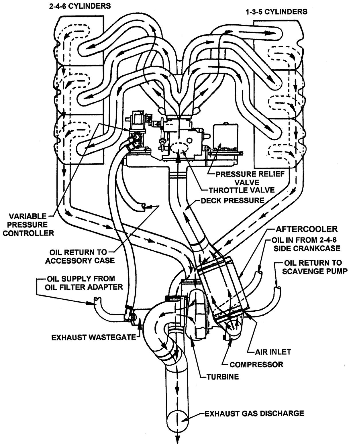
FIGURE 11-1. INDUCTION AND EXHAUST SYSTEM
