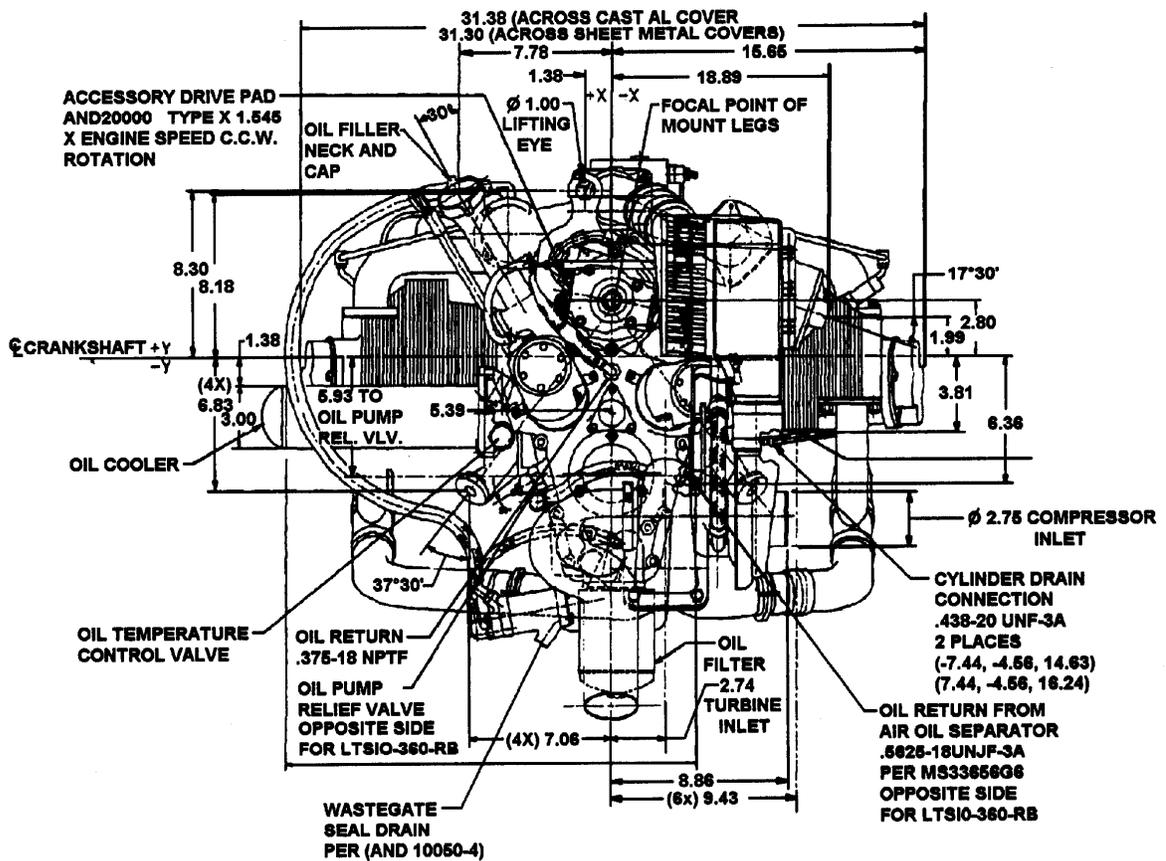
FIGURE 6-1. INSTALLATION DRAWING (cont'd)
