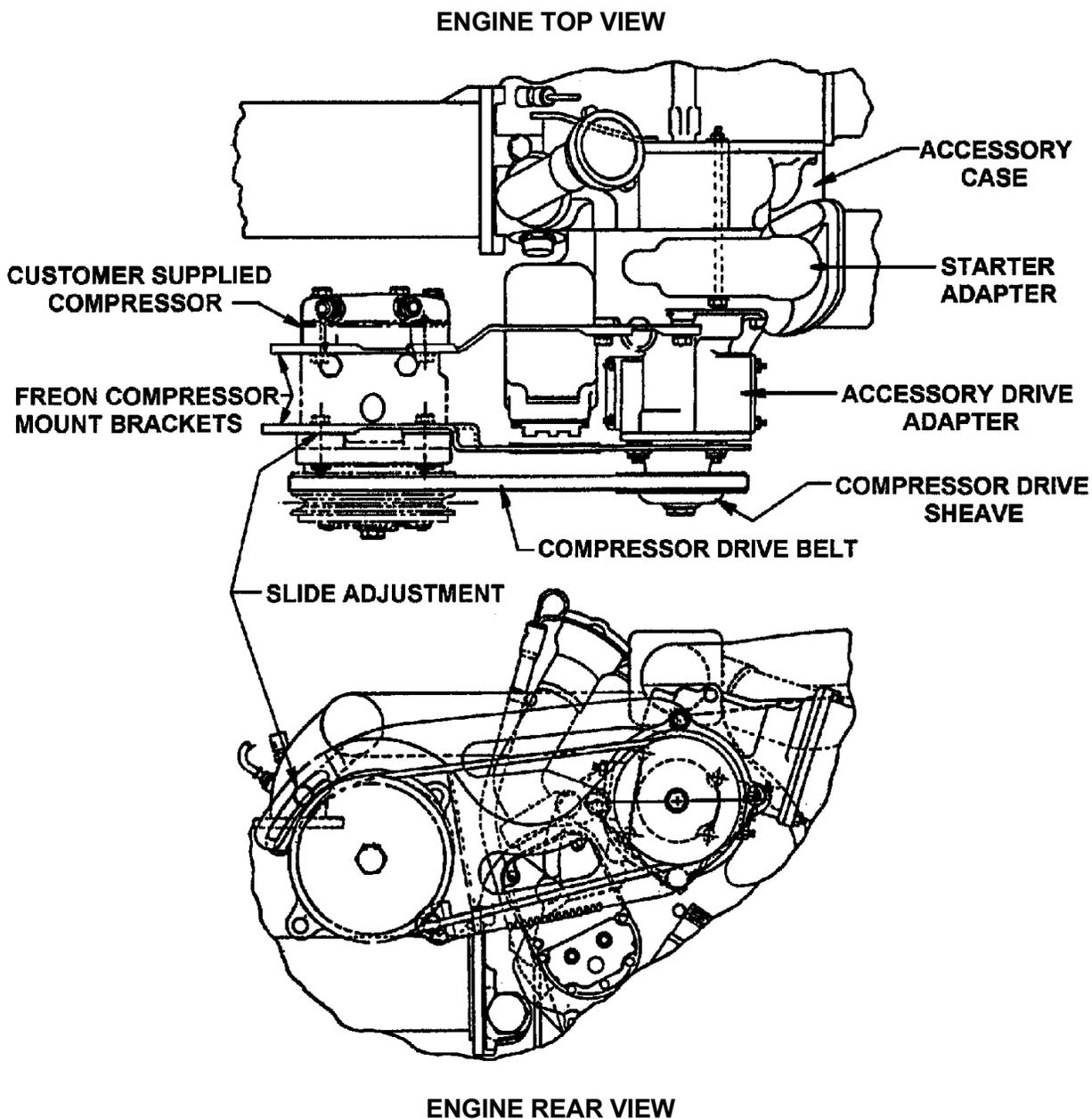
FIGURE 15-1. COMPRESSOR DRIVE (TSIO-360-RB)
