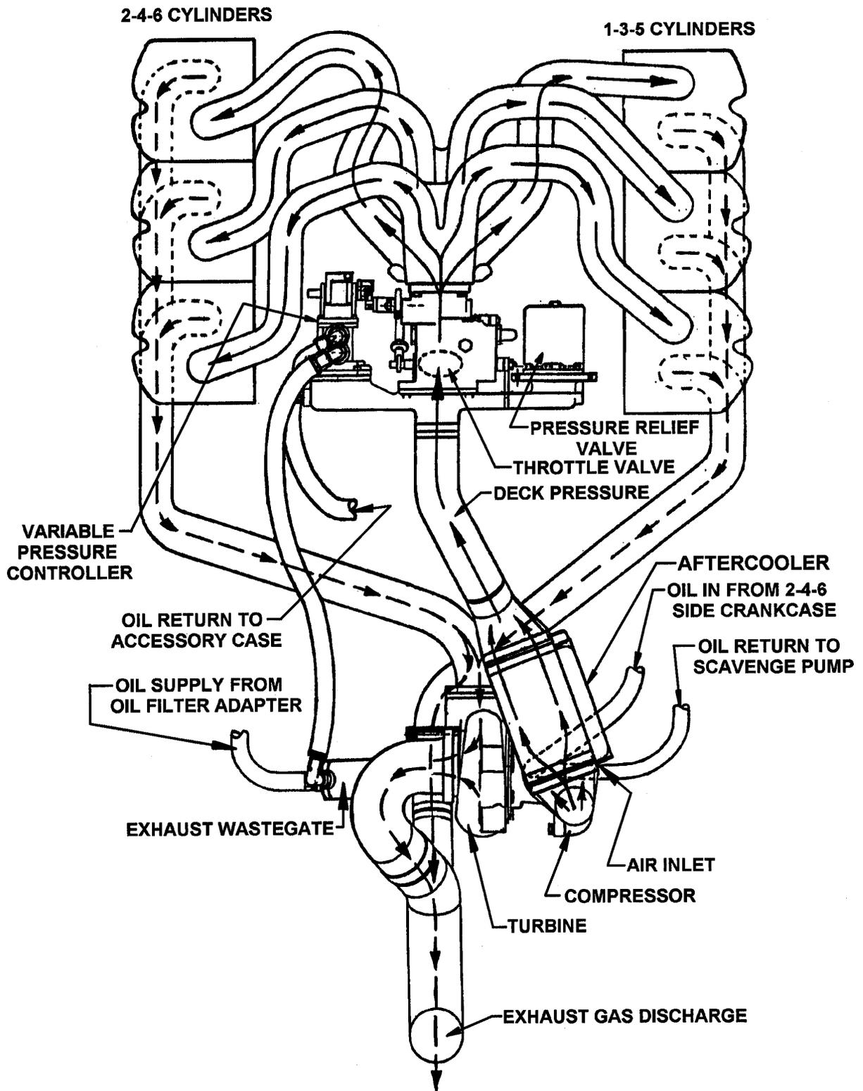
FIGURE 11-1. INDUCTION AND EXHAUST SYSTEM
