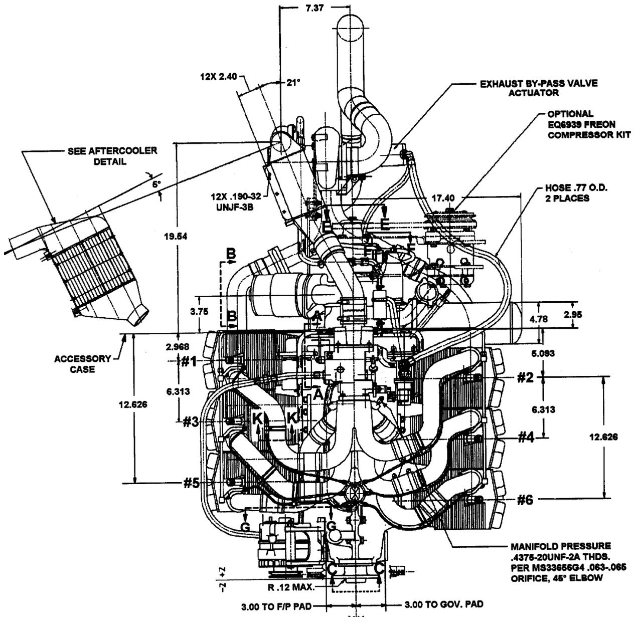
FIGURE 1-1. Engine Description L/TSIO-360-RB
