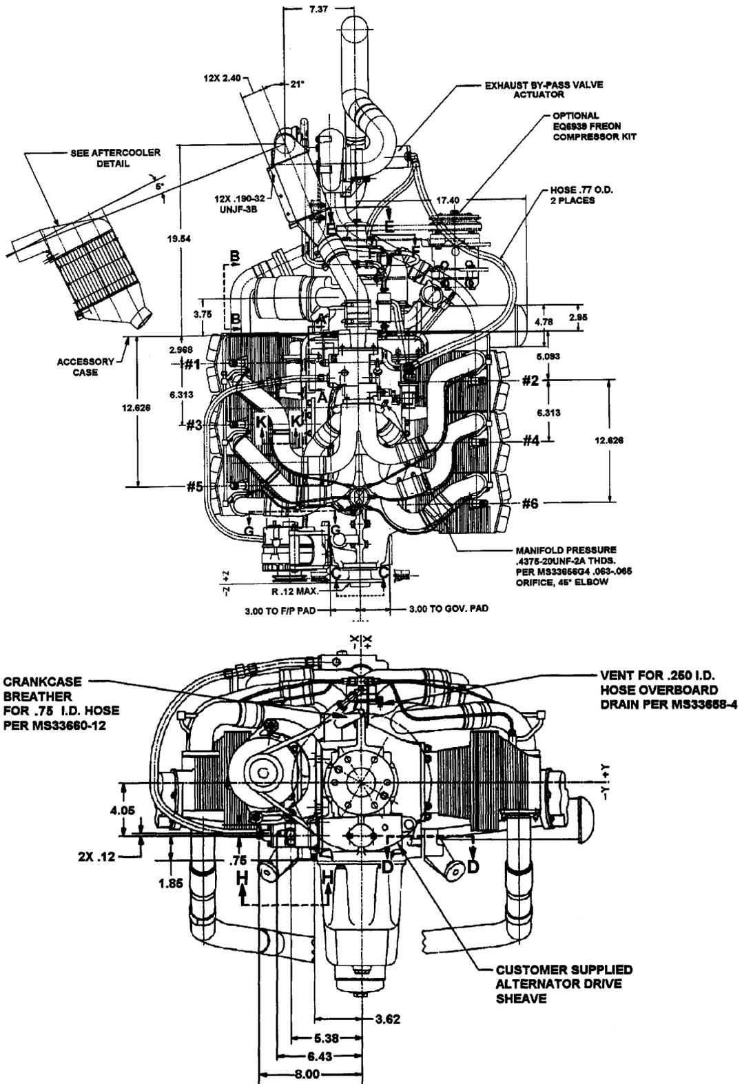
FIGURE 6-1. INSTALLATION DRAWING
