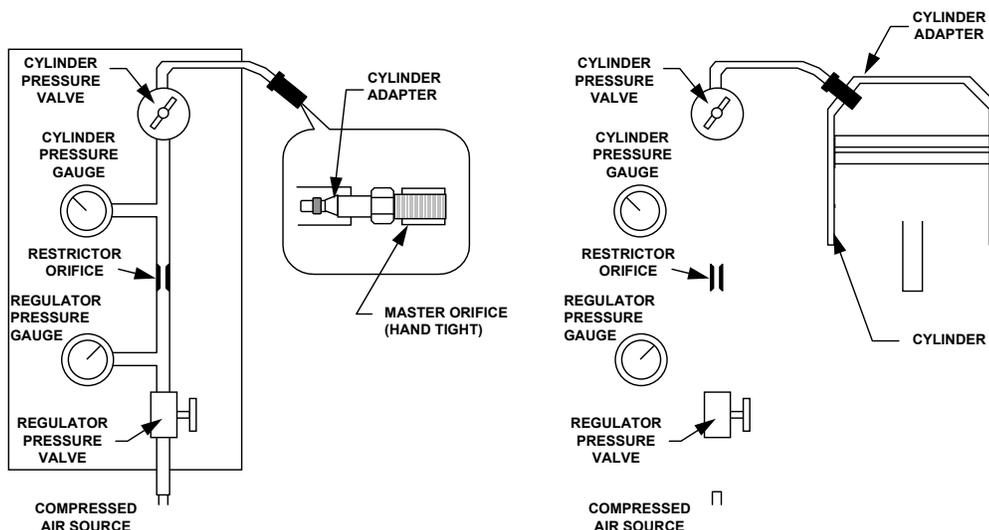
**FIGURE 20-10. DIFFERENTIAL PRESSURE TESTER CALIBRATION**
