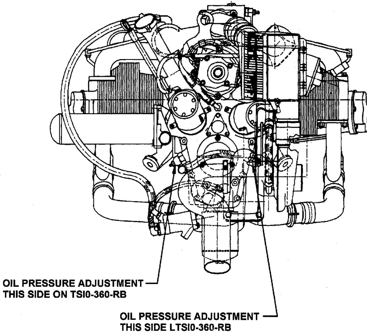
FIGURE 23-1. OIL PRESSURE ADJUSTMENT
