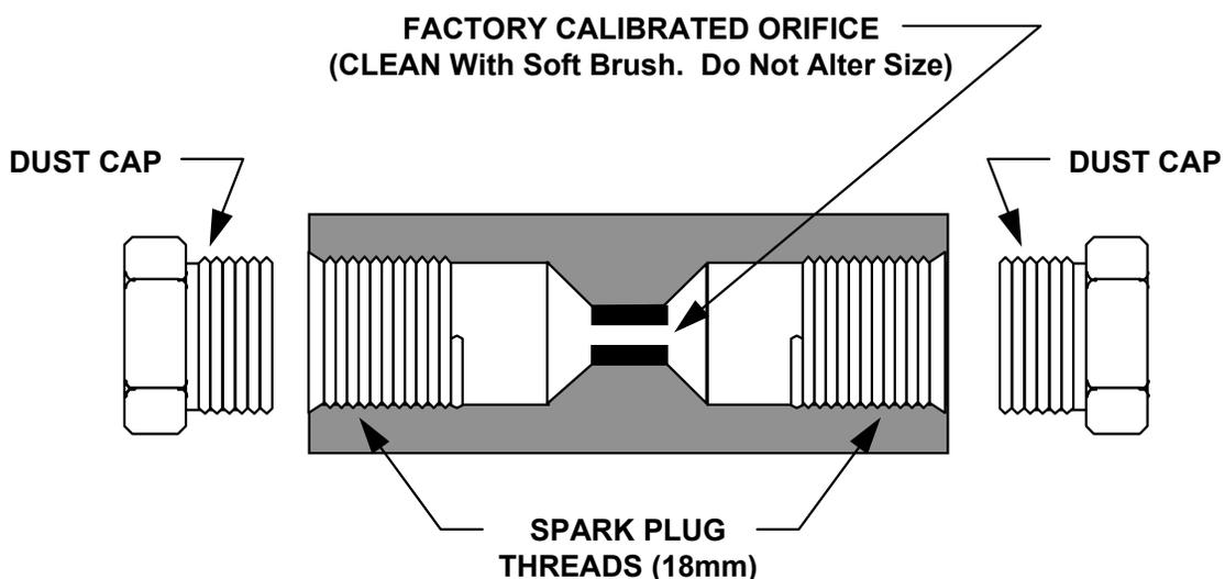
**FIGURE 20-7. MASTER ORIFICE TOOL (For procurement, see chapter 2)**
