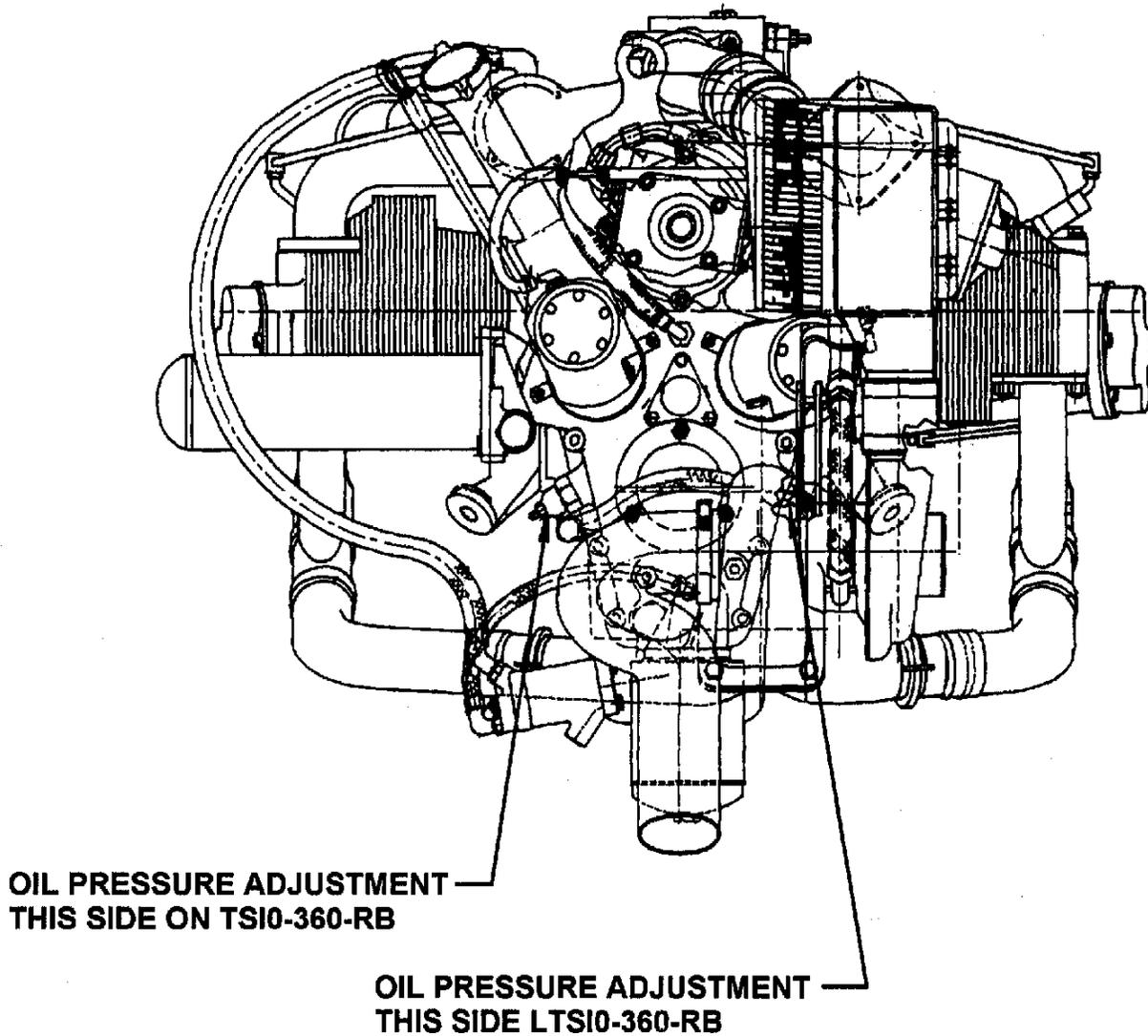
FIGURE 23-1. OIL PRESSURE ADJUSTMENT
