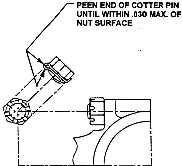
**FIGURE 4-5. CONNECTING ROD COTTER PIN INSTALLATION**
