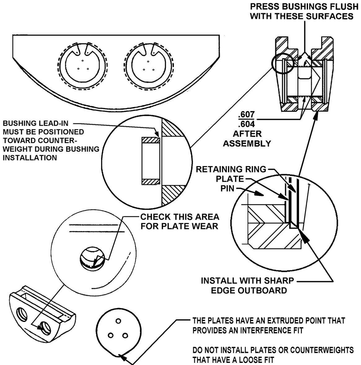
**FIGURE 18-4. COUNTERWEIGHT INSPECTION, REPAIR AND INSTALLATION**
