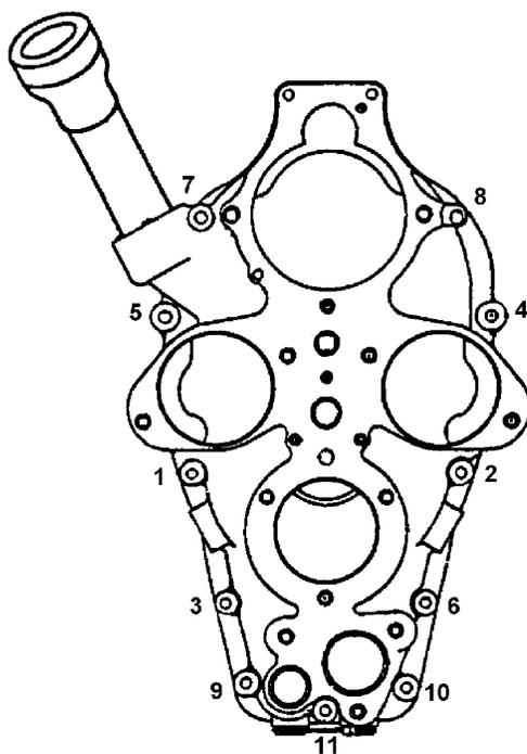
**FIGURE 19-12. ACCESSORY CASE TORQUING SEQUENCE**
