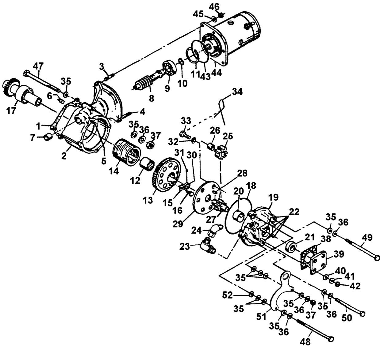
FIGURE 6-8. OPTIONAL STARTER ADAPTER ASSEMBLY (TSIO-360-RB)
