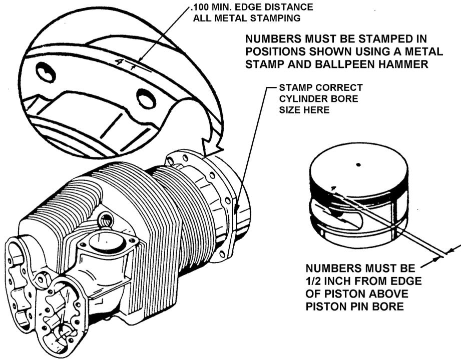
FIGURE 16-15. CYLINDER AND PISTON POSITION NUMBER
