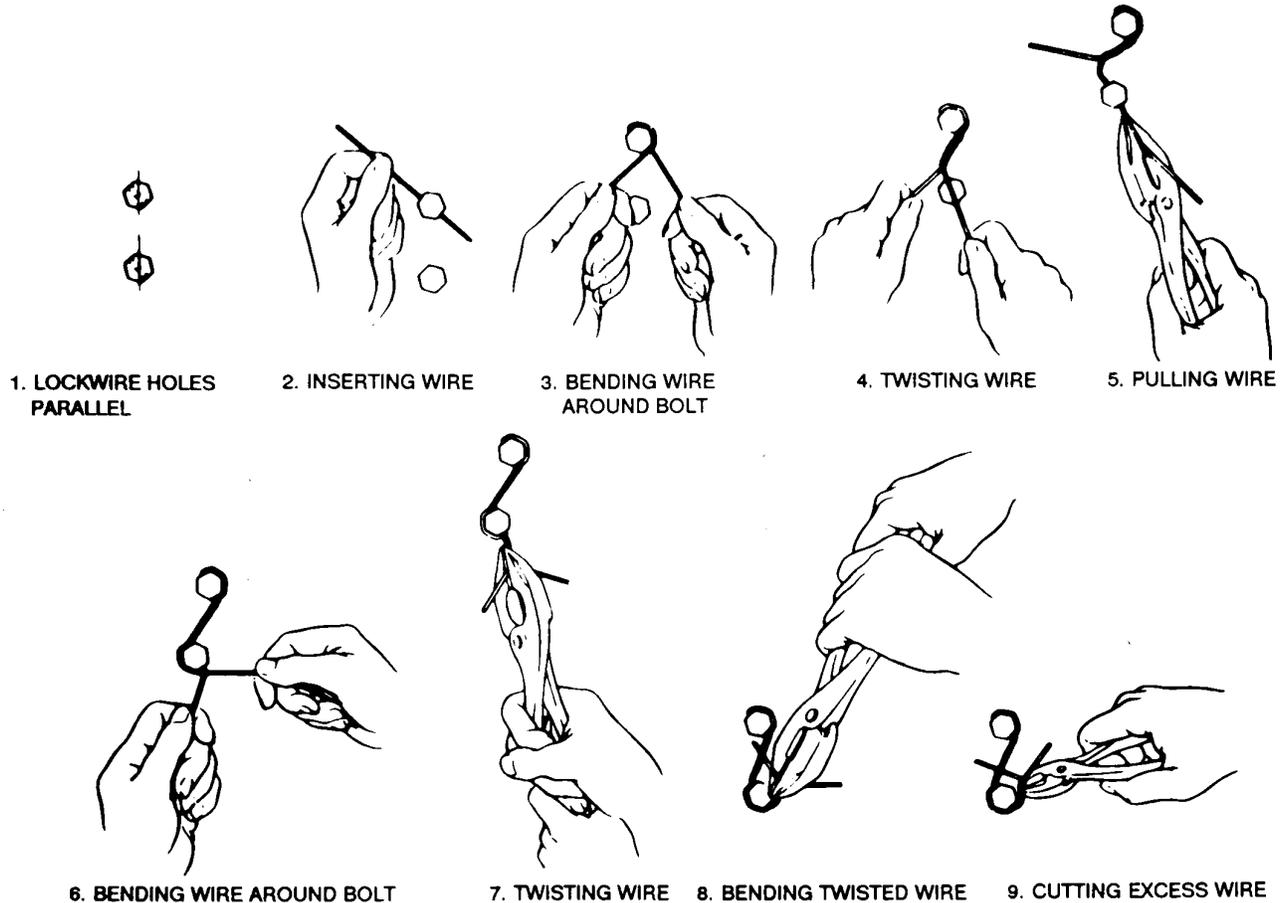
FIGURE 4-1. GENERAL LOCKWIRE PROCEDURE
