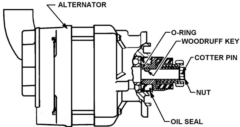
FIGURE 12-3. ALTERNATOR DRIVE COUPLING COMPONENT ASSEMBLY
