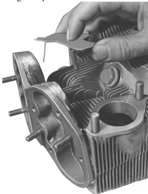
**FIGURE 16-17. INSTALLING BAFFLE**
