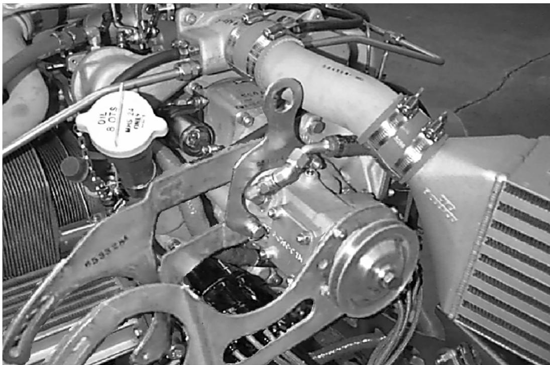
**FIGURE 19-13. GENERAL ACCESSORY CASE AND ACCESSORIES INSTALLED**
