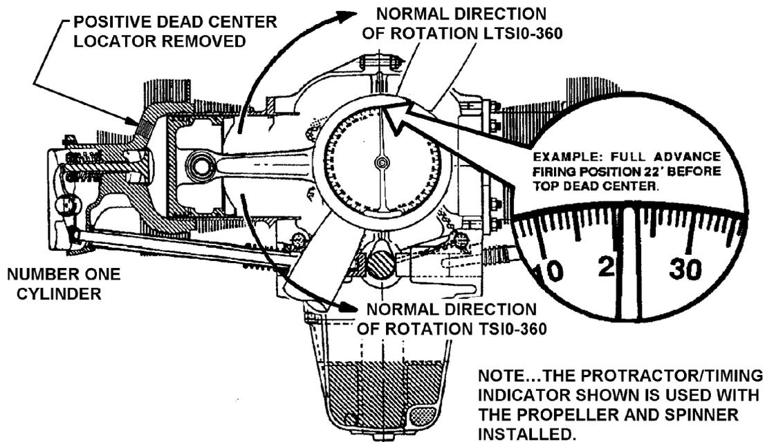
**FIGURE 19-24. TIMING POSITION STEP FIVE**
