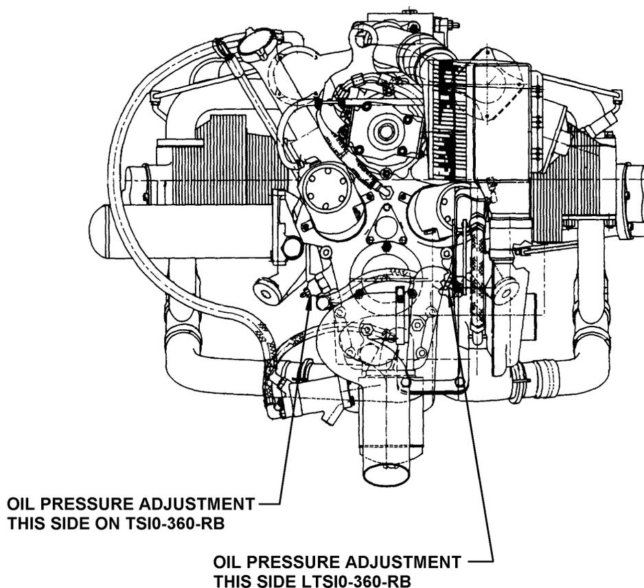
**FIGURE 20-1. OIL PRESSURE ADJUSTMENT**
