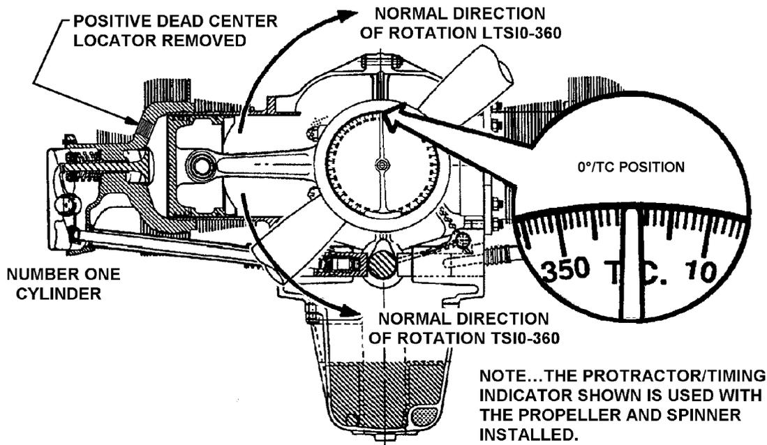
**FIGURE 19-23. TIMING POSITION STEP FOUR**
