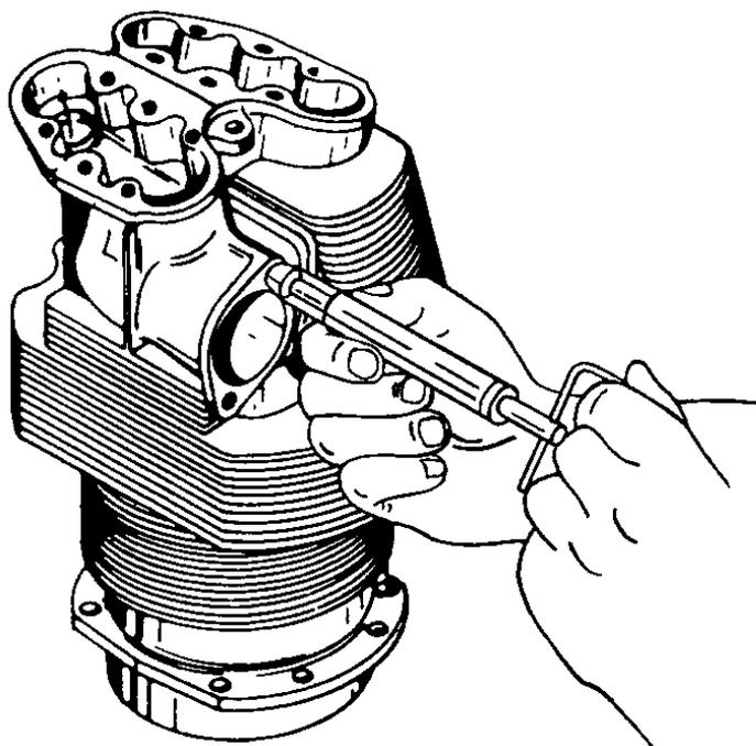
FIGURE 5-1. INSTALLATION TYPICAL HELICAL COIL INSERT
