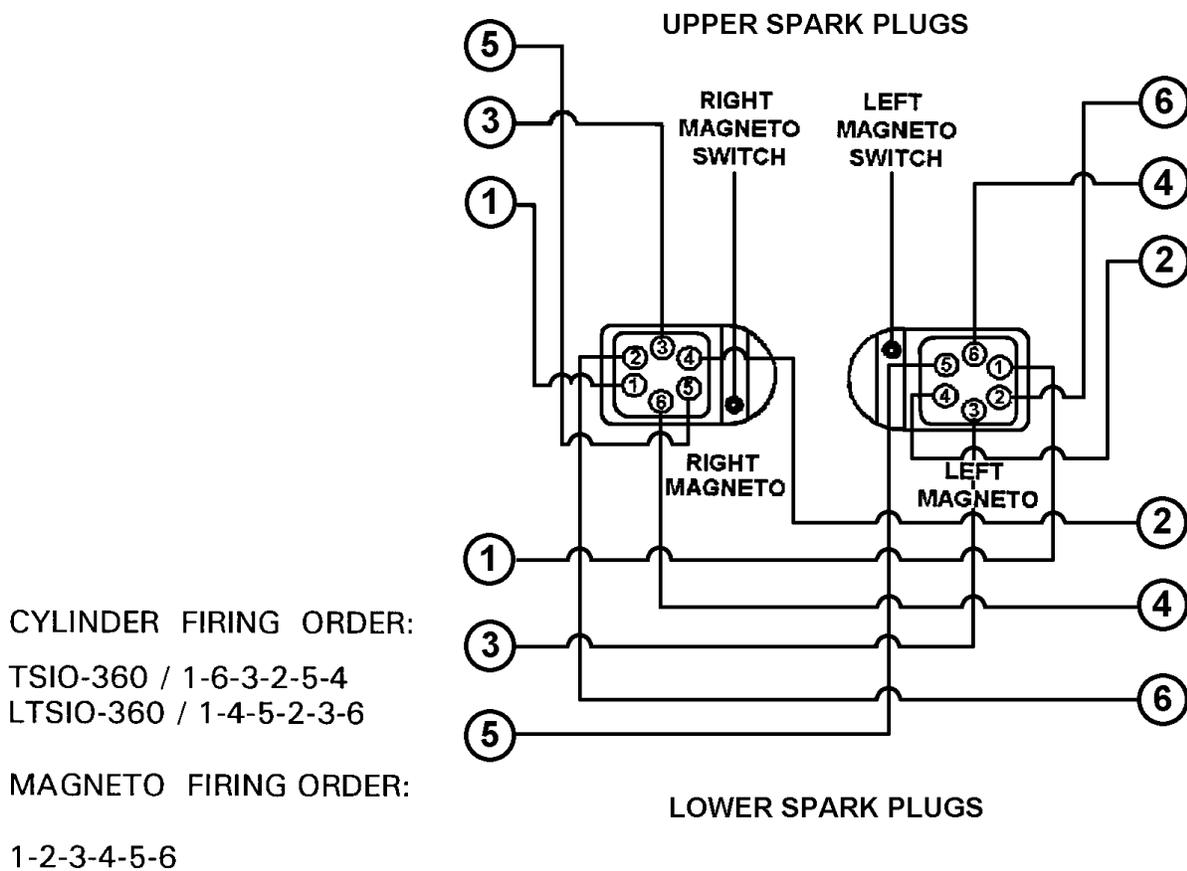
**FIGURE 19-26. IGNITION WIRING DIAGRAM**
