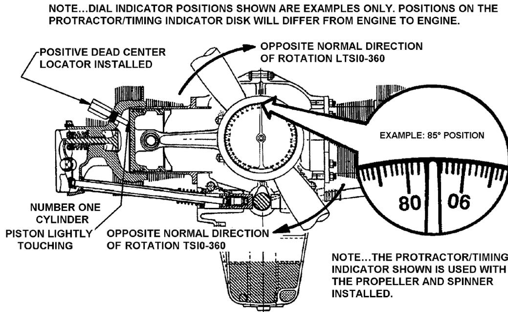
FIGURE 19-21. TIMING POSITION STEP TWO
