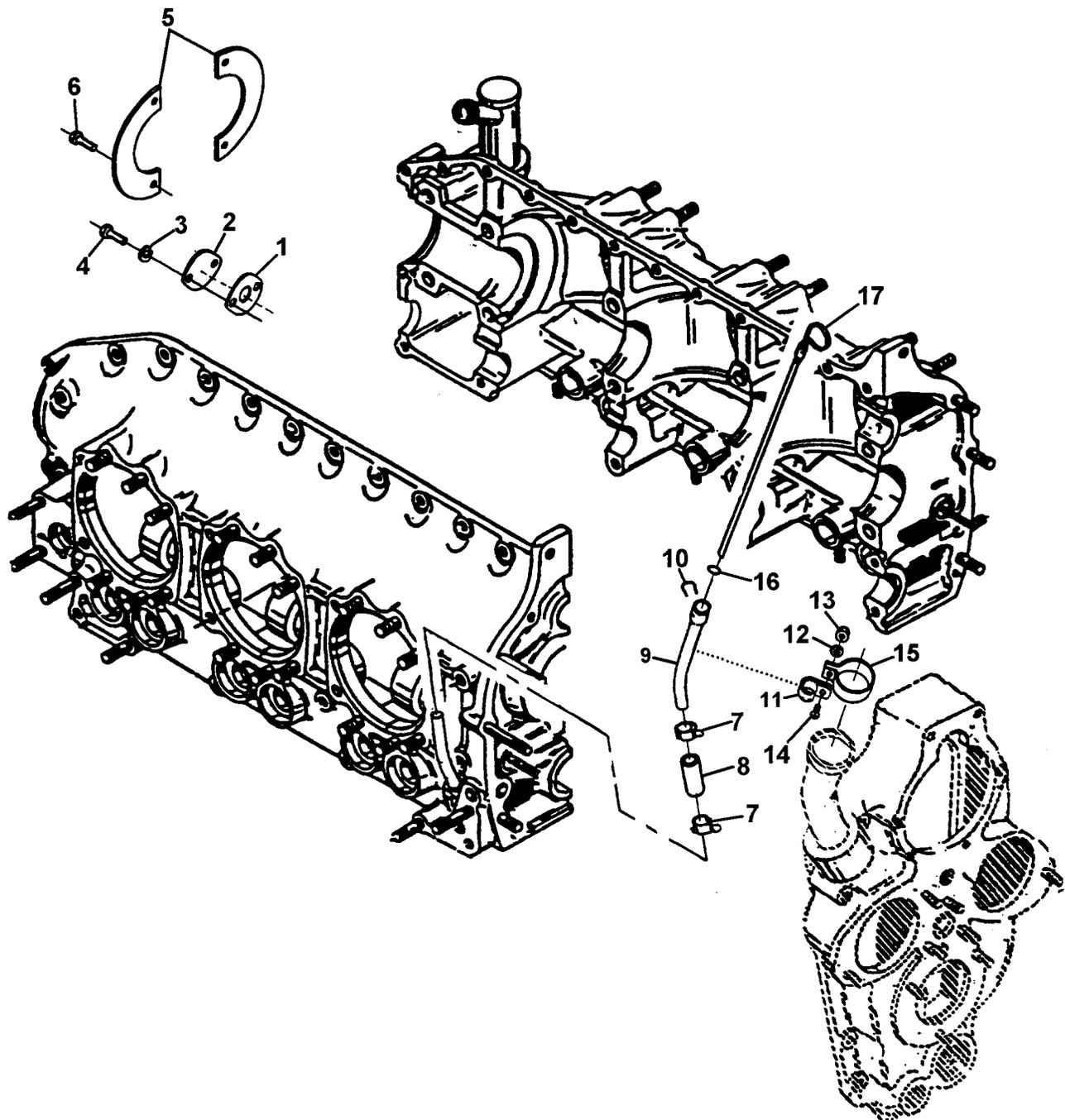
FIGURE 6-16. CRANKCASE ASSOCIATED PARTS
