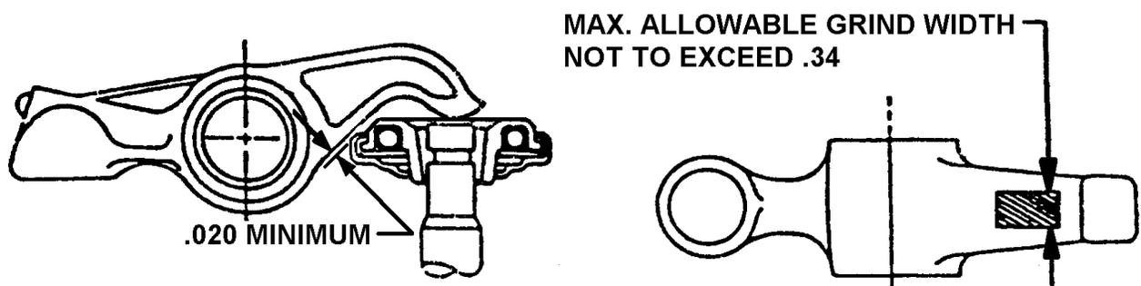
FIGURE 16-12. ROCKER ARM TO ROTOCOIL CLEARANCE
