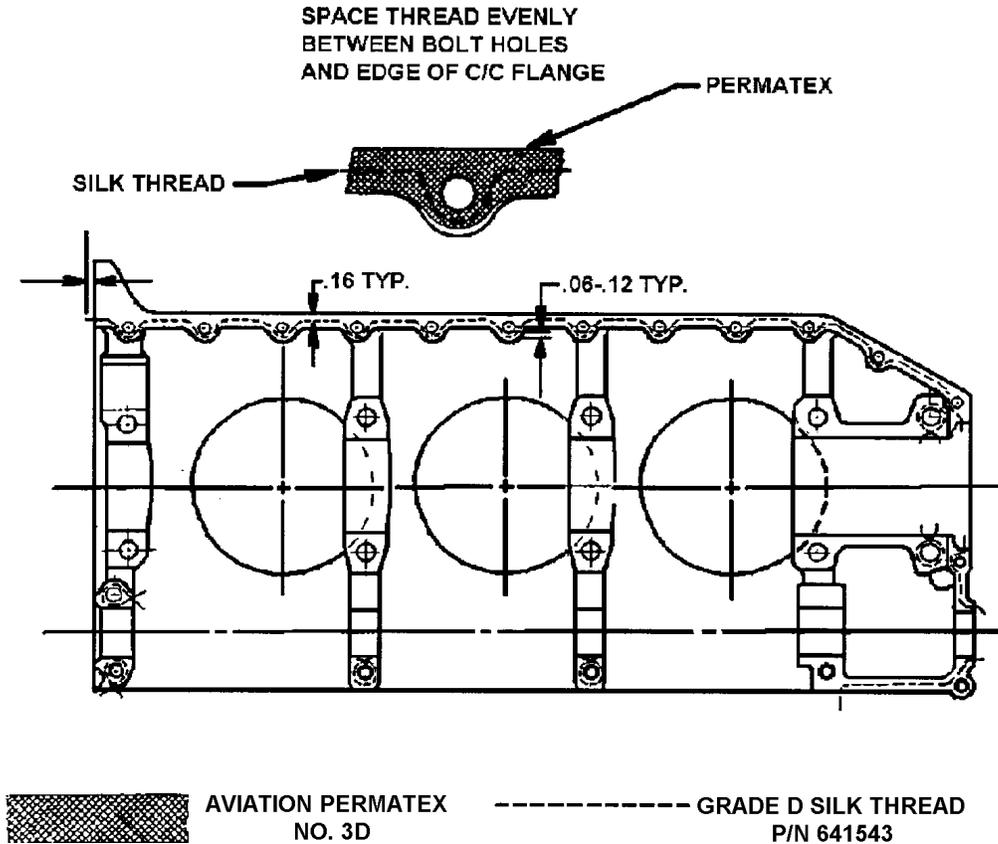
FIGURE 19-3. CRANKCASE SEALANT AND THREADING PROCEDURE
