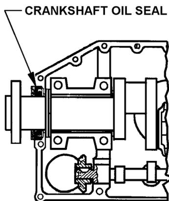
**FIGURE 19-5. CRANKSHAFT OIL SEAL INSTALLED**
