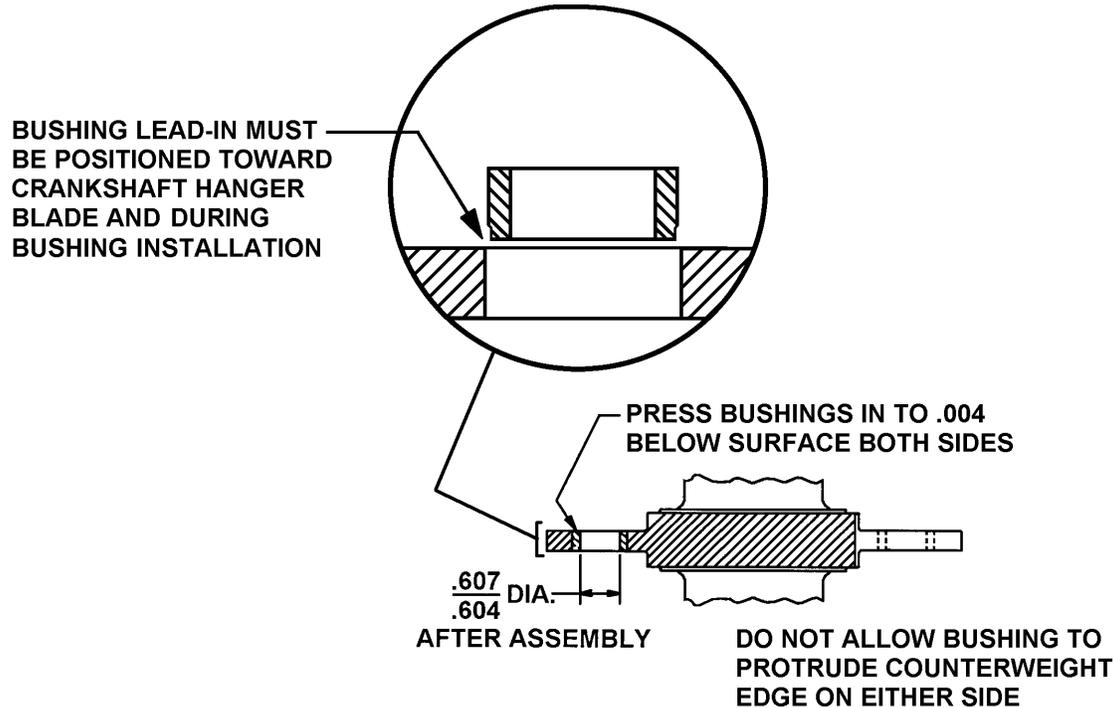
**FIGURE 18-3. CRANKSHAFT HANGER BLADE BUSHING REPLACEMENT**
