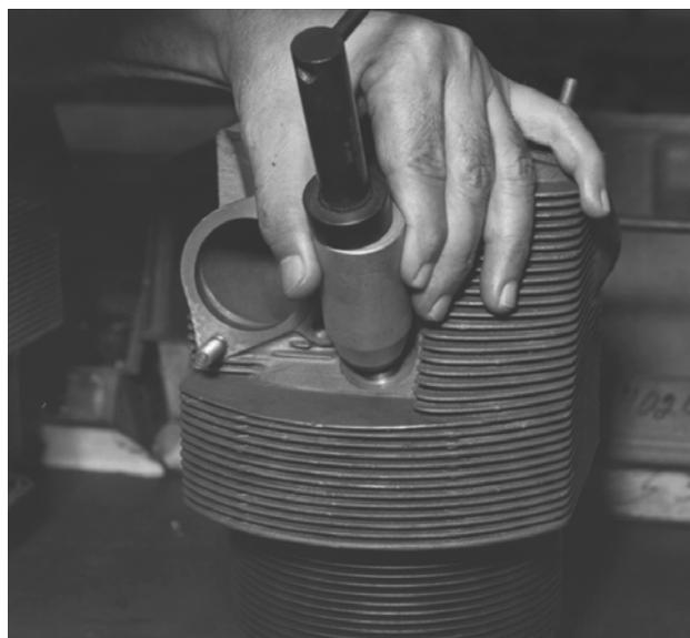
**FIGURE 16-9. INSTALLING SPARK PLUG HELICAL COIL**
