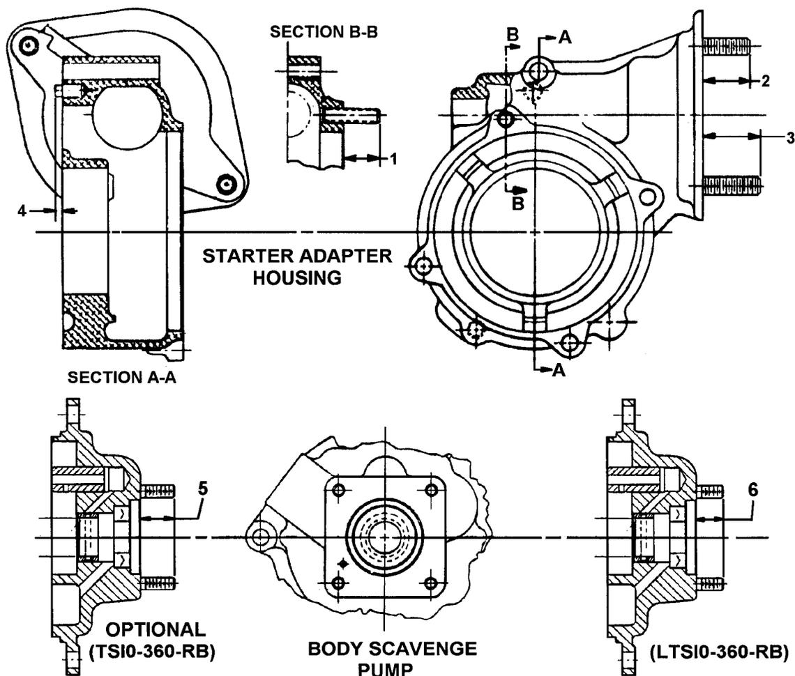
FIGURE 13-2. STARTER ADAPTER STUD SETTING HEIGHTS
