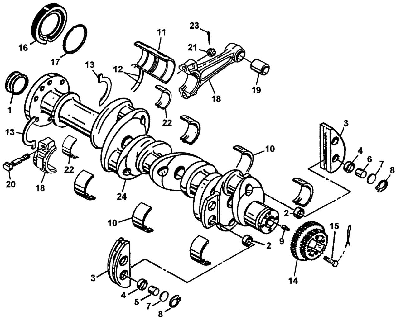
**FIGURE 6-19. CRANKSHAFT ASSEMBLY**
