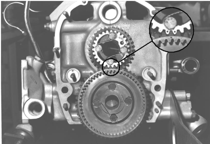
**FIGURE 19-2. ALIGNMENT OF TIMING MARKS**
