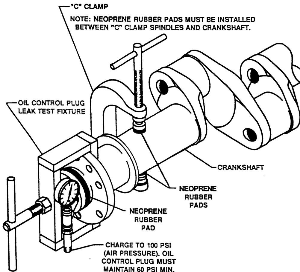
NOTE: FIXTURES MUST BE INSTALLED CAREFULLY TO PREVENT CRANKSHAFT DAMAGE.
