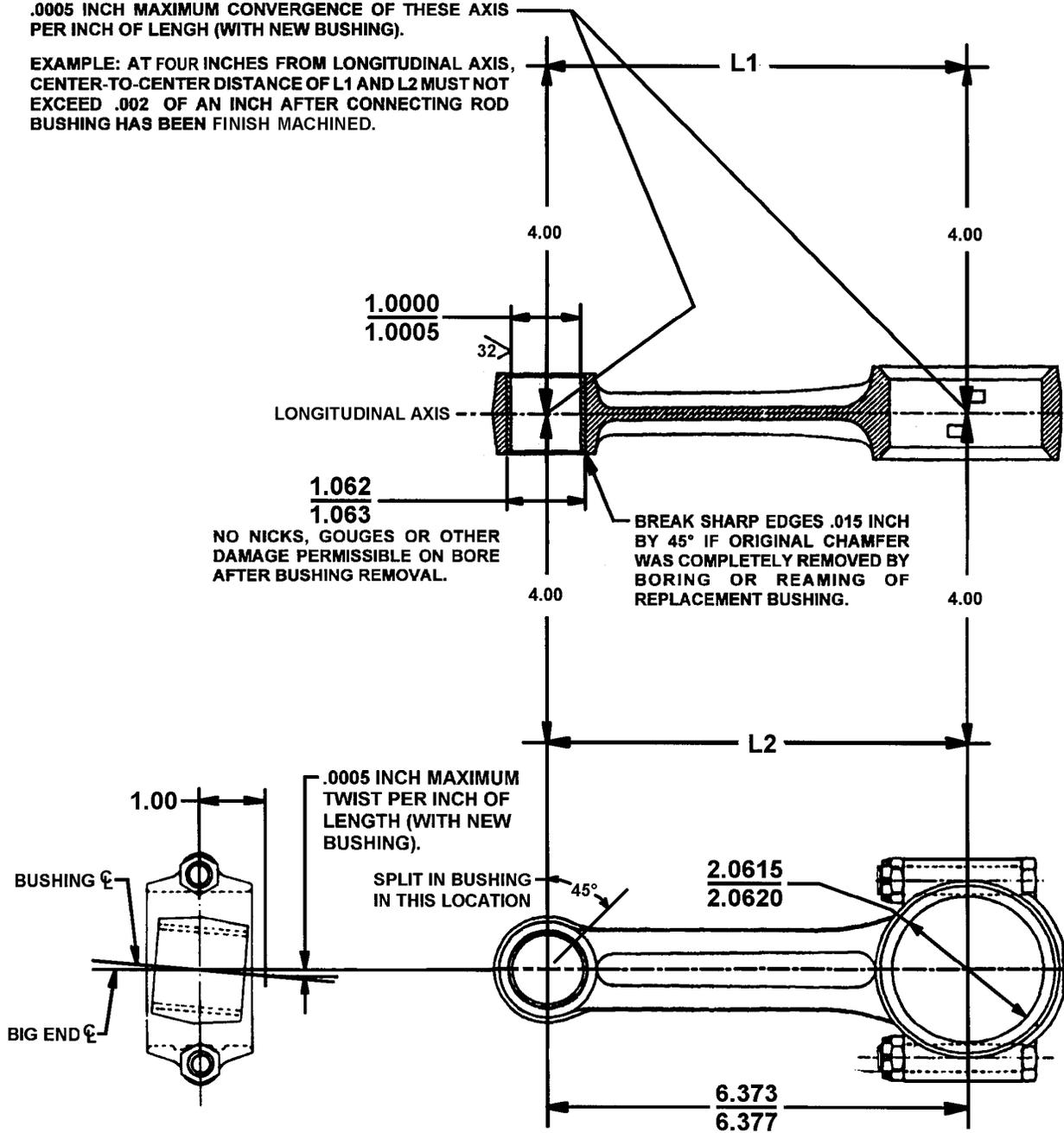
**FIGURE 18-2. CONNECTING ROD FITS AND LIMITS**
