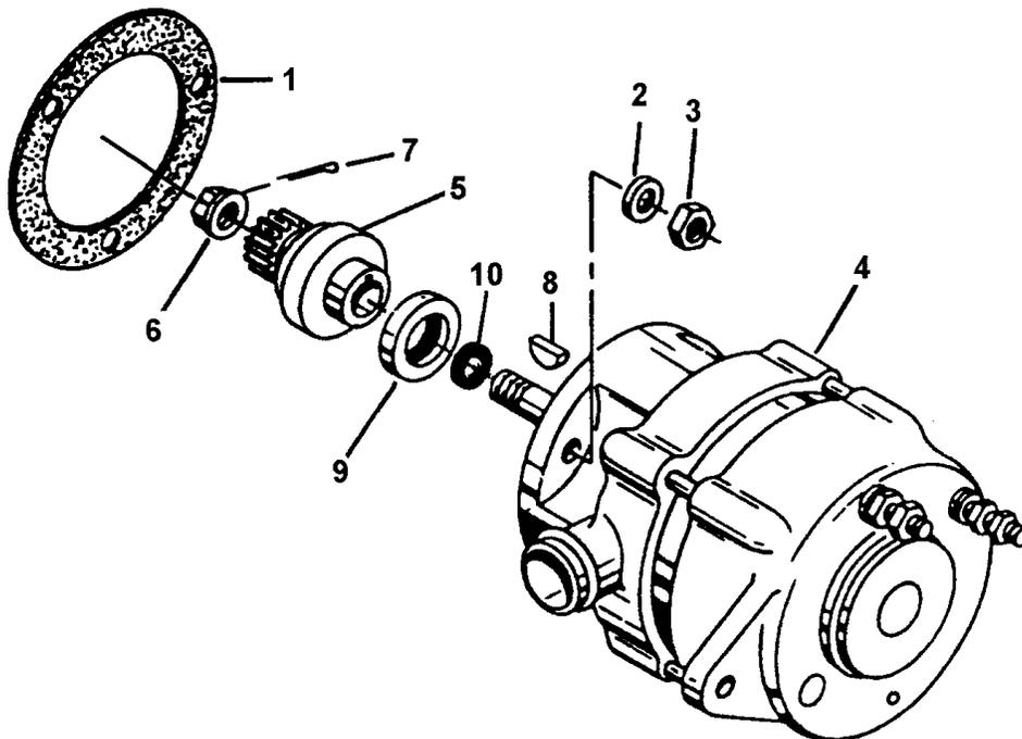
FIGURE 6-7. ACCESSORY CASE MOUNTED ALTERNATOR ASSEMBLY
