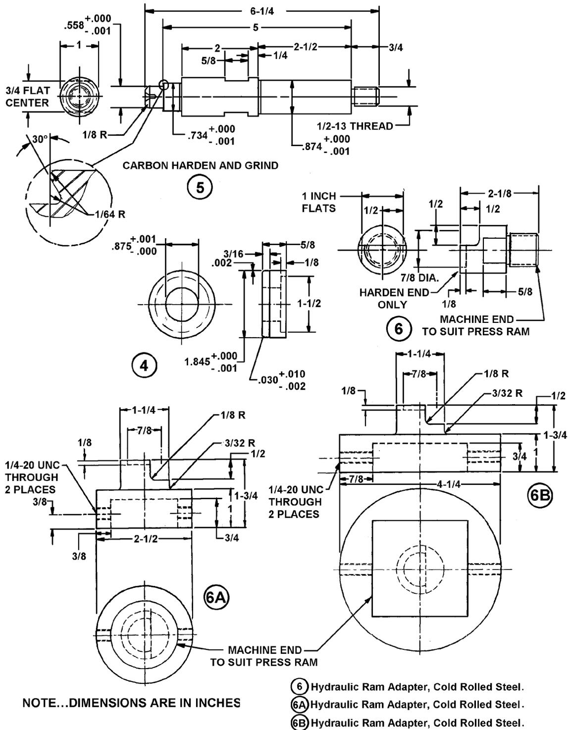
FIGURE 11-3. STARTER ADAPTER NEEDLE BEARING INSTALLER (continued)
