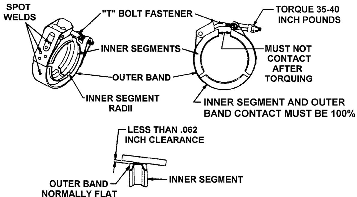
FIGURE 19-19. MULTI-SEGMENT "V" BAND CLAMP
