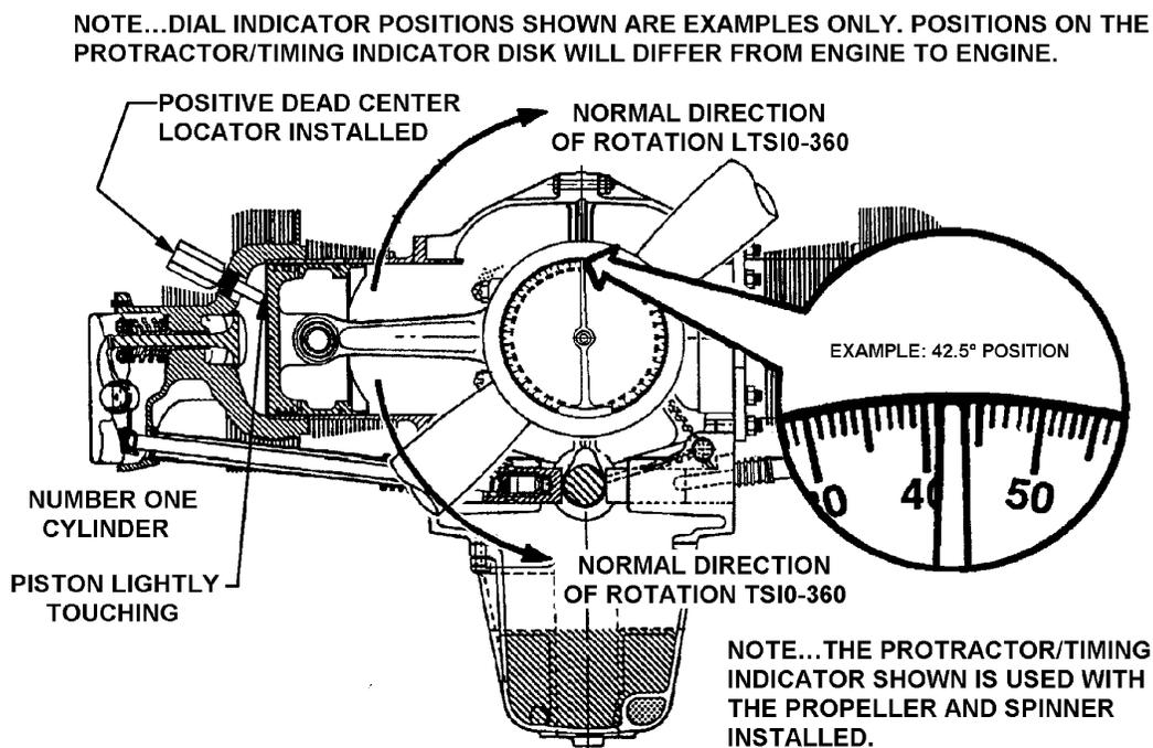
FIGURE 19-22. TIMING POSITION STEP THREE
