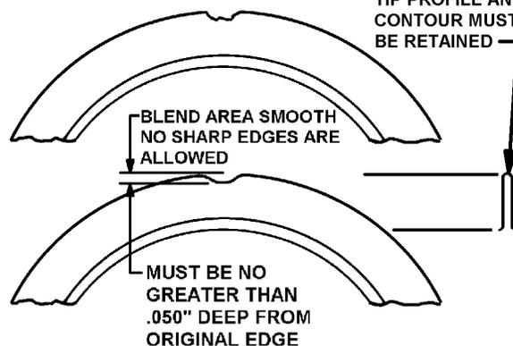
**MAGNETIC PARTICLE INSPECT REPAIRED AREA FOR CRACKS AND IF NONE ARE PRESENT, APPLY PROTECTIVE COATING OF TCM ENAMEL OR EQUIVALENT**
