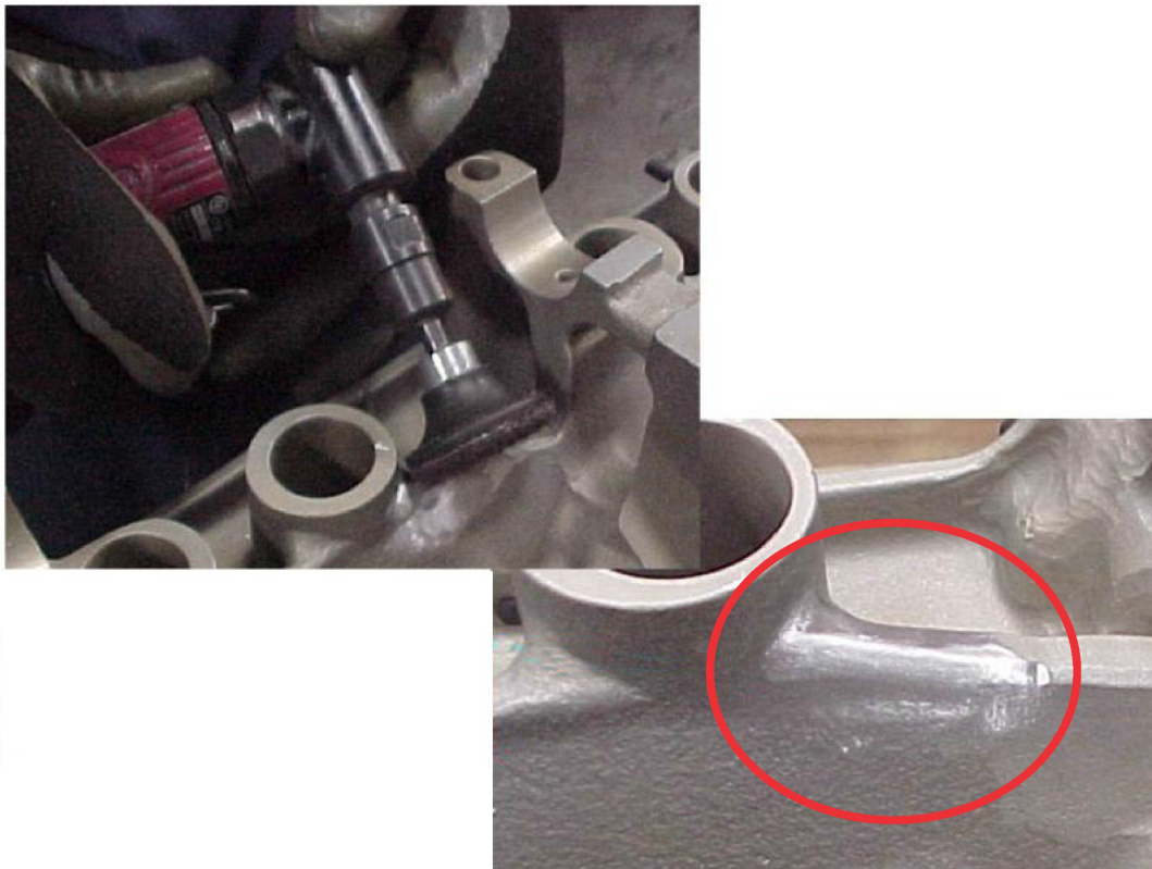
Figure 7. Crankcase Finished Surface, deburring
