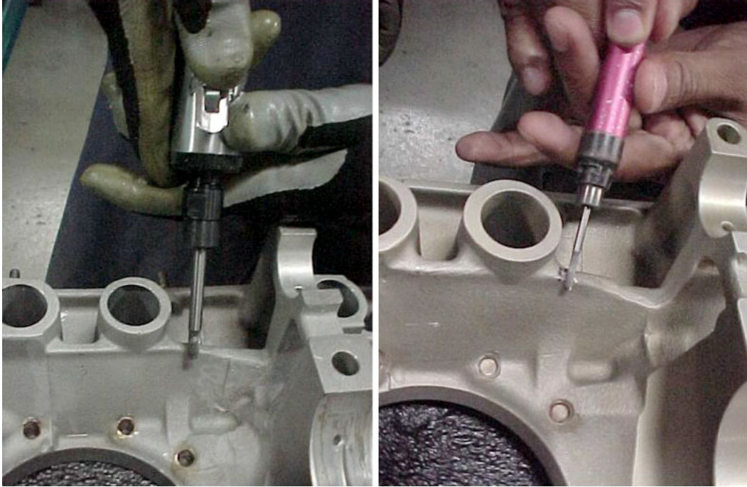
Figure 5. Crankcase Clearance Modification, typical
