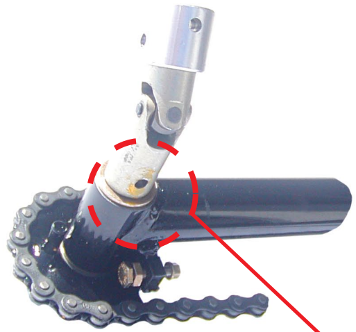
TAPER PIN REMOVED VIEW B
